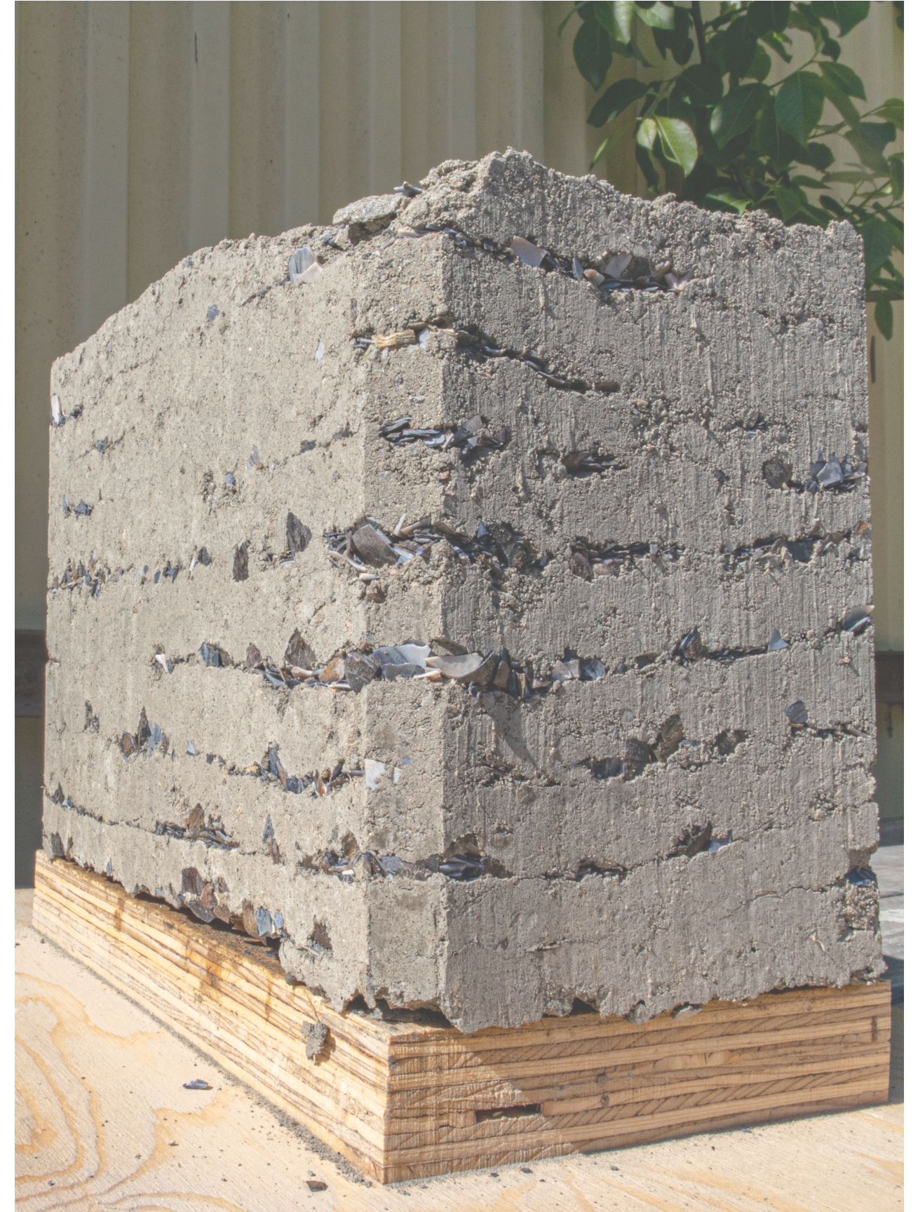
Gothenburg Rammed - testing the local earth mixture adding crushed blue-mussels as layers in a rammed earth prototype. The idea wast to create a local material identity by adding layers of mussels as an ornament, but it could perhaps also have effects on preventing erosion. No pigment was added in the mixture, the photo shows the rammed earth block after drying for a couple of days.
