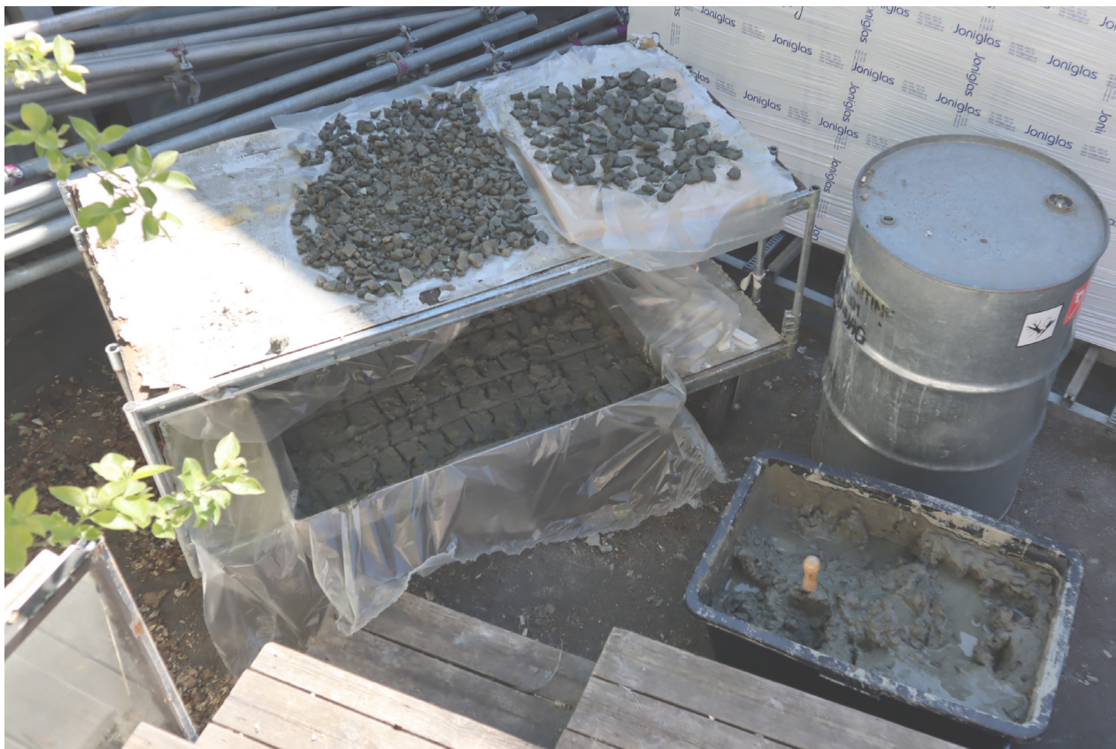
The Clay process - image showing the drying process of the wet waste-clay
