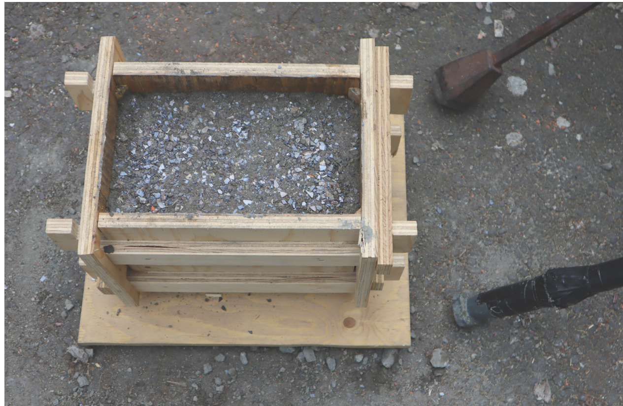
Blue Mussels - The idea of adding blue mussels into the clay mix is explored, relating to the cities marine heritage and Fiskekörkan located by the station. A part from the aesthetics the mussels/shells could improve the insulation, structural aspects properties of the Rammed Earth elements. There is potential in the mixing and ramming process to introduce new layers of bio-based material.
