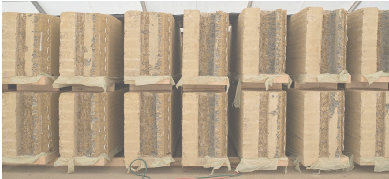
Figure 11. Image of the pre-fabricated elements cut on site(Halbe, 2019).
