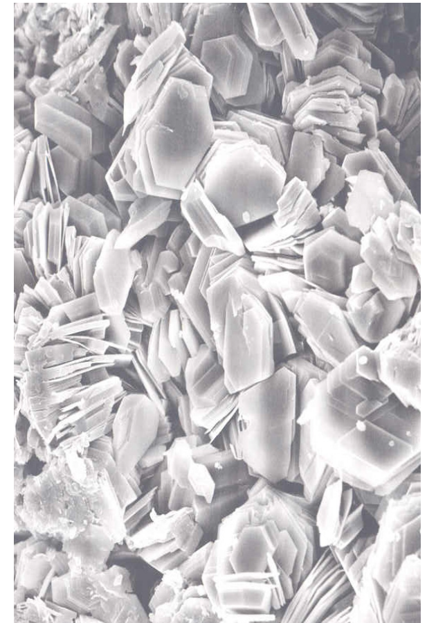
Clay – the most important component in rammed earth Image of Kaolinite Clay – Scanning Electron Microscope (© 2004 PetroTech Associates)
