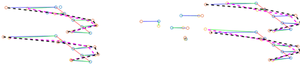
Figure 8.6: Third Mode Shape Comparison: EMA and FEA of Pre-calibration Model
