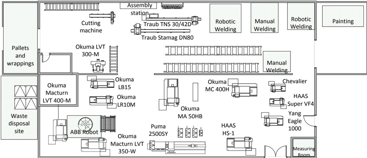
Figure 1 - Factory layout over the production area.
