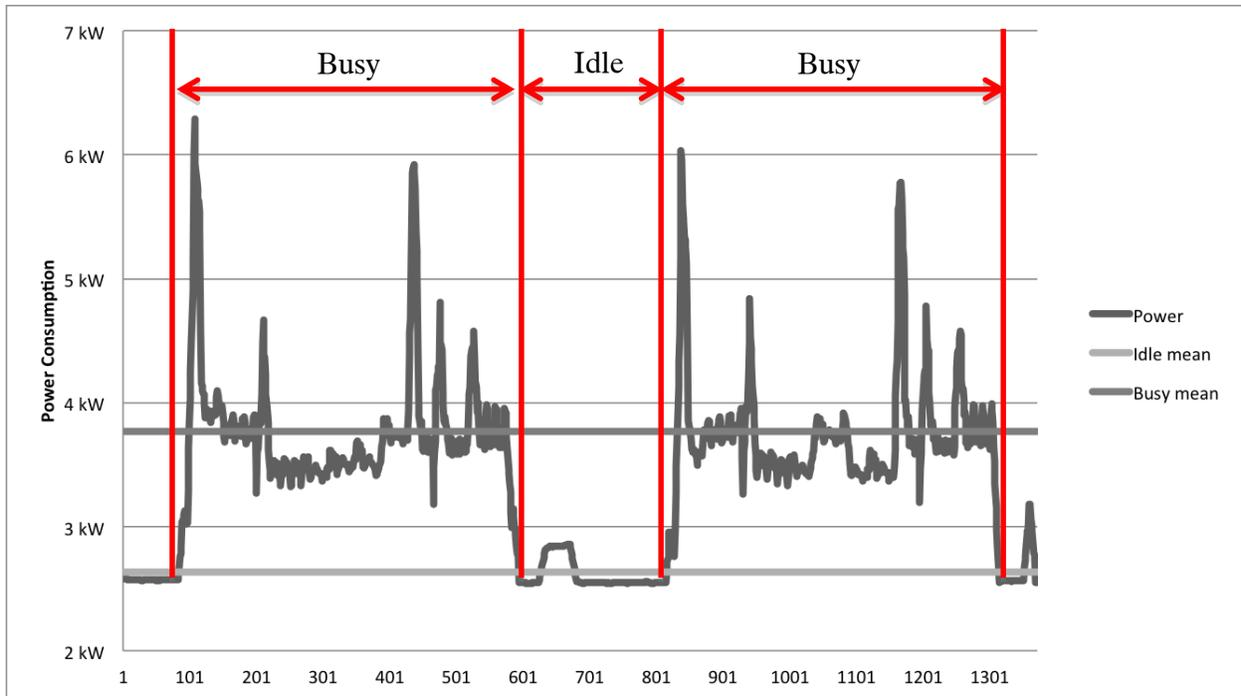
Figure 8 - Energy consumption for Okuma MC400H.
