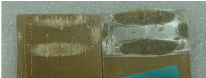
Figure 4.6: Welding with 471 Ampere
