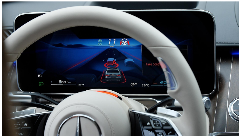
Figure 5. The button on the steering wheel will display a red light when Drive Pilot requires the driver to take over the driving task
