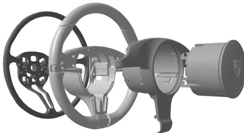
Figure 2: Exploded view of a steering wheel (Porsche 997 II) (Harrer & Pfeffe, 2017)
