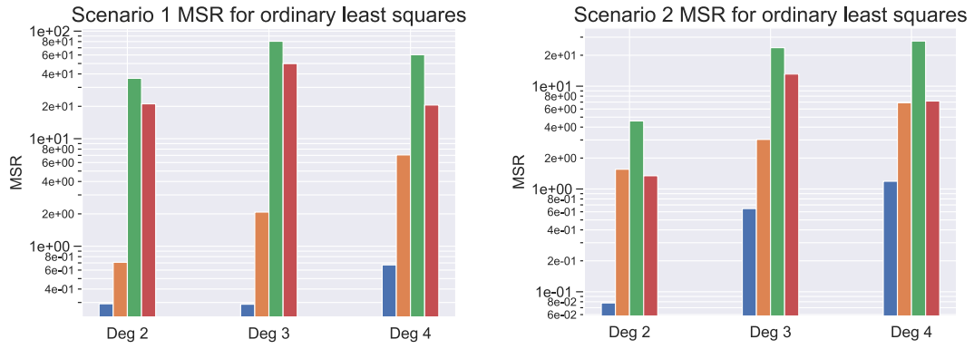
Figure 15: MSR of R_p for OLS models of varying orders for scenarios 1 and 2. The MSR for A1, A2, A3 and B2 are represented in blue, orange, green and red respectively.
