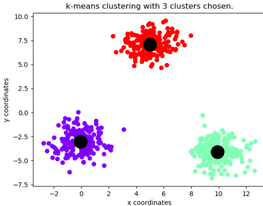
Figure 2.5: k -means clustering on three blobs of data is shown in this figure. The larger black points represent the three cluster centers calculated by the k -means clustering algorithm.
