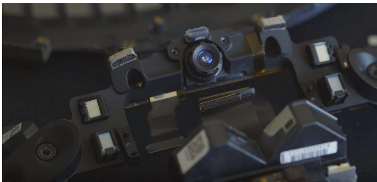
Figur 2.9 Sensorer i HoloLens
