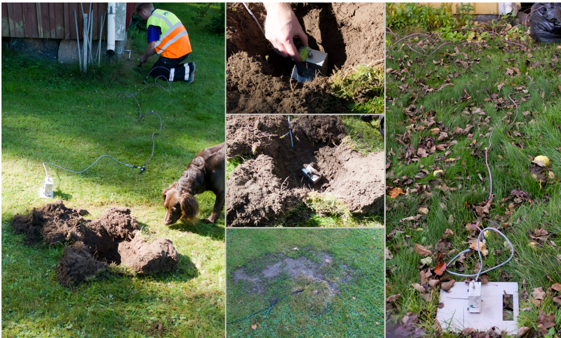
Figure 3.1: Left: Trigger geophone at foundation and hole for ground geophone. Middle: Leveling the geophone (top), partly covered geophone (middle) and refilled whole with dug down geophone (bottom). Right: Leveled geophone on steel plate placed on lawn and triggering geophone on foundation in the background of the picture.
