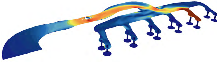
Figure 4.26: Velocity chart of the NACA design with adiabatic temperature as a boundary condition on the cylinder head wall with valve 2 open.
