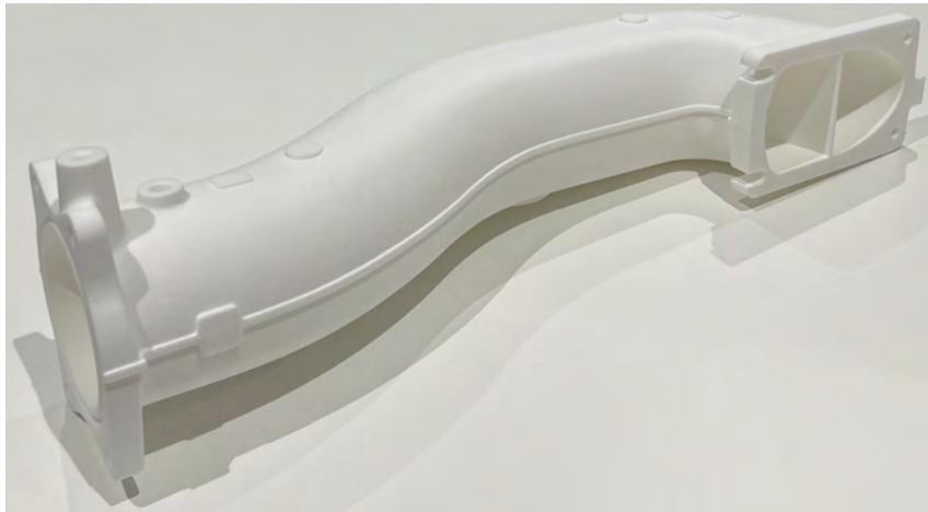
Figure 4.30: Picture of the final 3D-printed prototype of the NACA with a vane.
