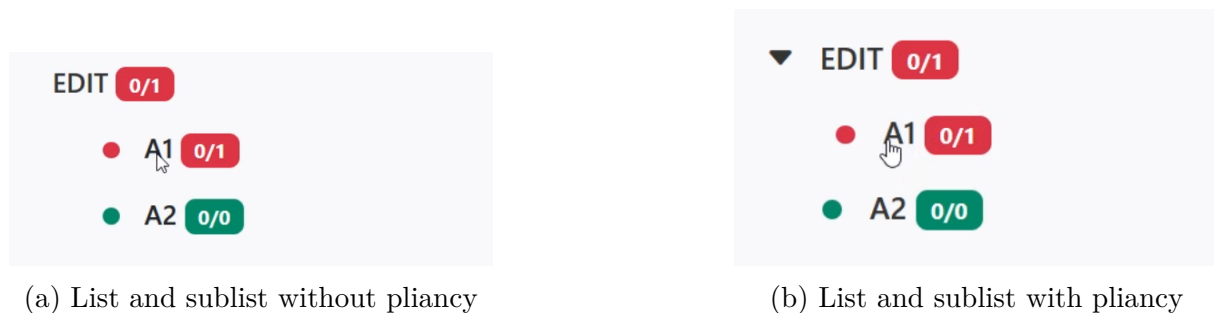
Figure 14: Comparison of a list and sublist design. (a) shows a static version without any interactive visual cues. (b) includes pliant design features such as a toggle-able triangle icon, subtle animations, and cursor changes on hover, indicating interactivity and improving usability.
