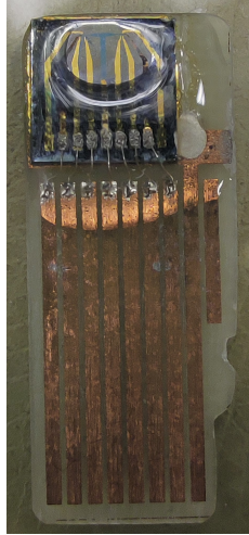
Figure 2.2: Two G-FET's fitted on a SD-card carrier
