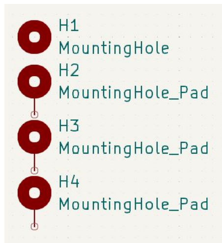
Figure B.11: Four mounting holes to attach the PCB to something.
