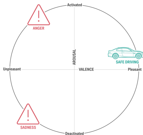
Figure 4.1: Driver state taxonomy based on Russel’s circumplex arousal-valence model [2] and the Yerkes-Dodson law [3]. Positive valence and medium arousal values have been shown to be the desired states in driving [4]
