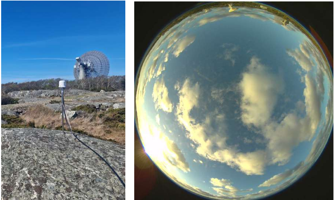
Figure 3.5: Image of sky camera near the Weather Station, as well as an example image from its archive.
