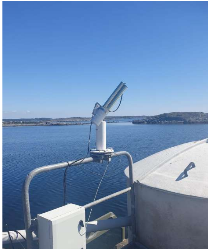
Figure 3.2: The AERONET sun-photometer at the OSO.
