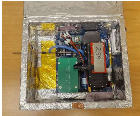
Figure 3.6: Image of the POPS instrument in one of its protective boxes.
