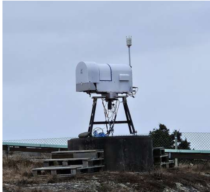
Figure 3.3: The HATPRO microwave radiometer on-site at the OSO.
