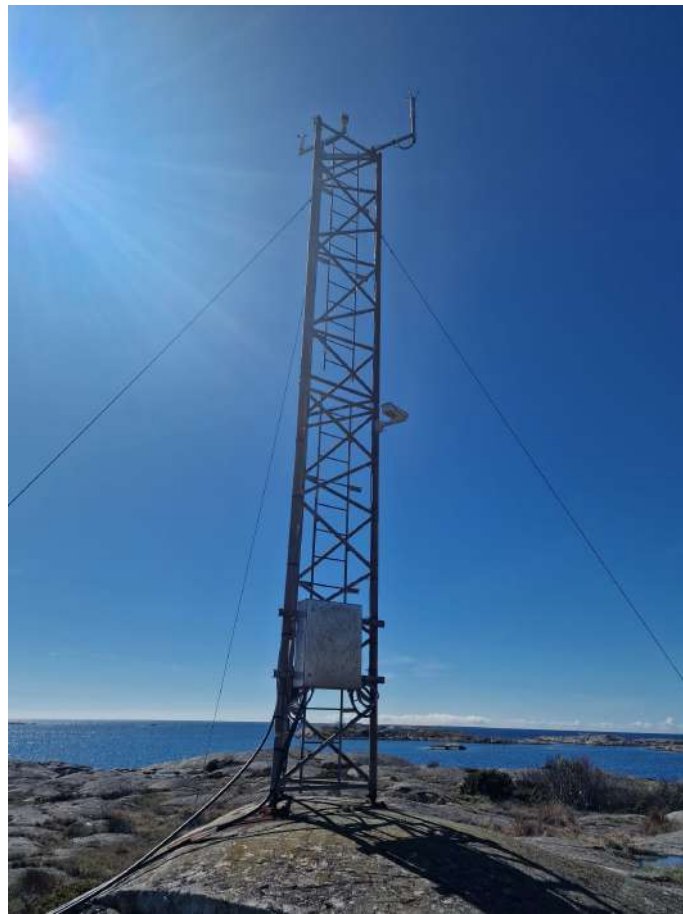
Figure 3.4: The weather station located at the OSO.
