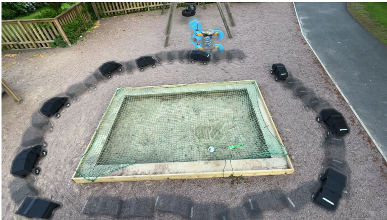
Figure 4.10: WM-RL following a path in large-grained sand going forwards. Left: Motion trail. Right: Birds eye view plot with blue as the original path to follow, green the adjusted path windows which the controller followed and in black its trajectory.
