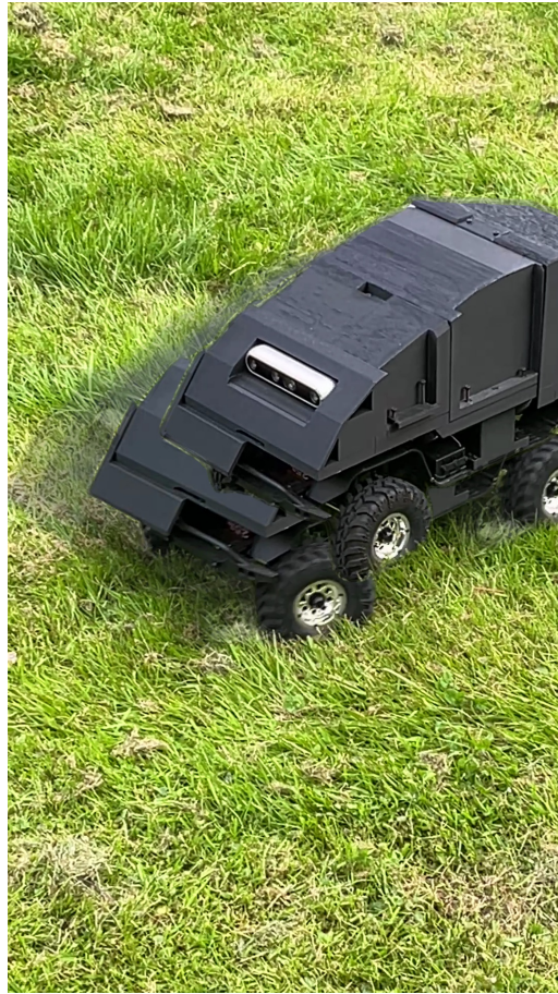
Figure 4.12: Orientation correction via reverse motion. The vehicle enters the frame from the right while turning right in the ego-centric frame. It then reverses while slightly turning left, before continuing forwards with an adjusted heading.
