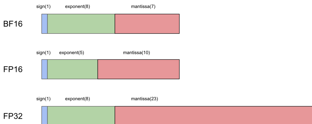
Figure 2.9: BF16, FP16 and FP32 formats. Different bit ranges for above three floating number representations.
