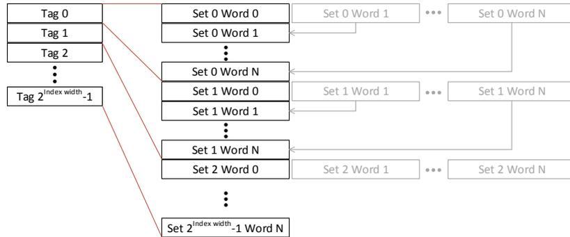
**Figure 4.2:** Implemented instruction cache memory block organization. The number of data words per line in a way is denoted by  $N$ .
