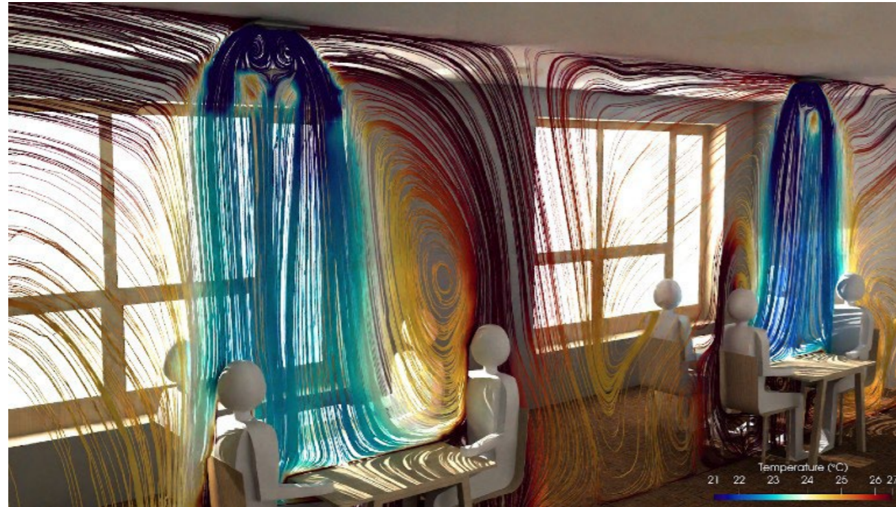
Figure 1. Temperature colored streamlines showing the fresh air intakes supplying air to the room (Khan, N 2021). CC-BY.
