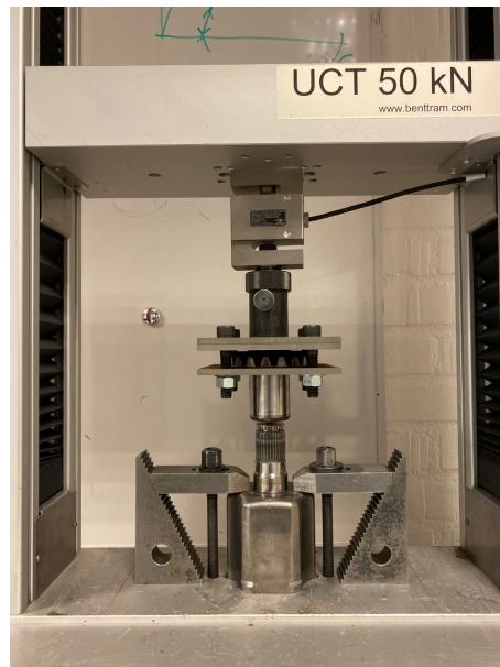
Figure 4.18: Assembly and disassembly set up in the UTM
