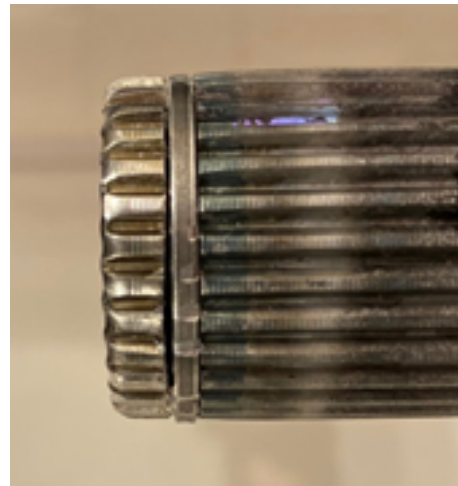
Figure 4.34: Visible damage on the third damaged shaft and dents on the ring
