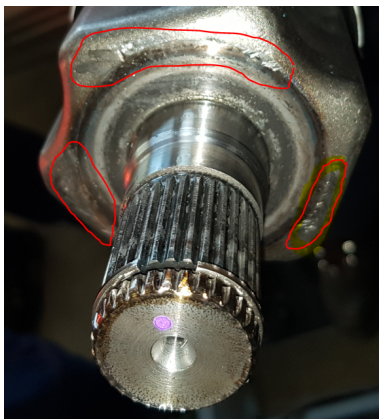
Figure 4.9: Marks on the shaft after disassembly
