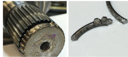
Figure 4.13: Damage on the shaft and ring after disassembly
