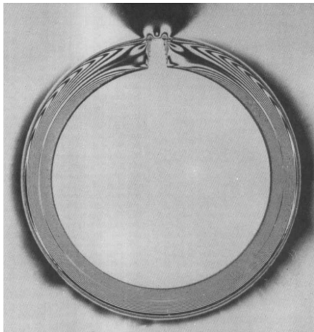
Figure 2.4: Stresses on a split ring compressed into a housing taken from [7]
