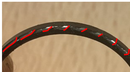
Figure 4.29: Contact marks on the surface of a ring after testing
