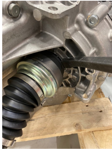
Figure 4.17: Lever used to dismount the shaft and support against the T-Roc gearbox housing
