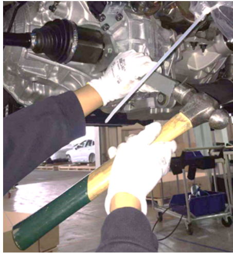
Figure 4.8: Shaft disassembly method using the wedge tool
