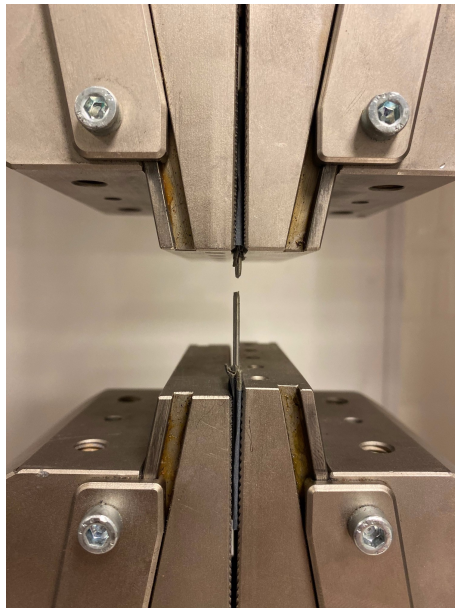
Figure 4.4: Tensile test on an unbent snap ring
