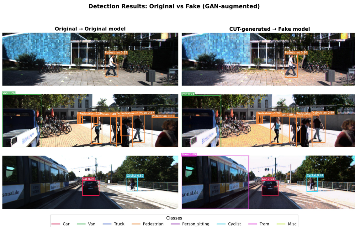
Figure 5.7: Detection results: original-trained model (left) versus style-transfer-trained model (right).
