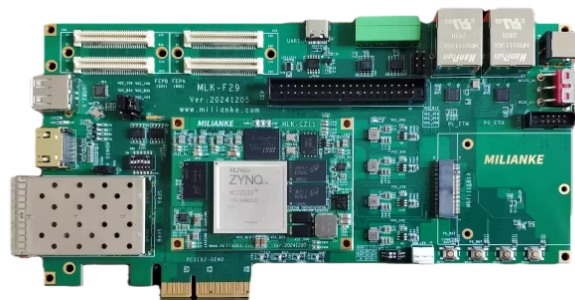
Figure 2.5: F29_CZ10_7035 development board with Xilinx Zynq xc7z035.
