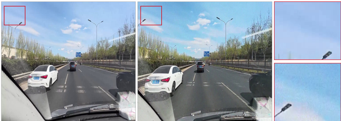
Figure 5.1: Visual comparison under normal daylight conditions. Left: DJI Action 5 Pro reference, center: system output, right: zoomed comparison of the marked region (DJI above, system output below).
