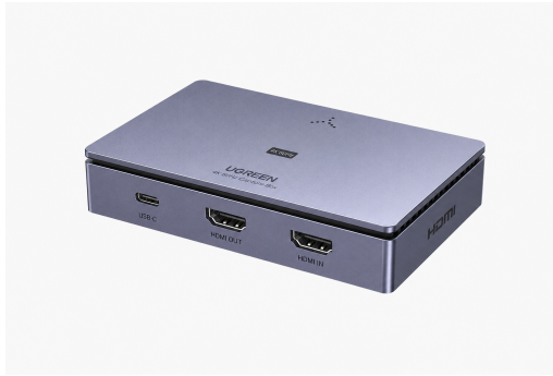
Figure 2.8: Video capture card used for HDMI-to-USB conversion.
