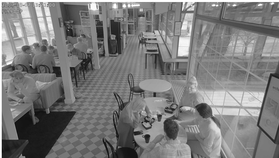
Figure 4.16: The IR-camera is at a low angle from the ceiling at Stena Center, which results in people being partially covered and their faces possibly obstructed.
