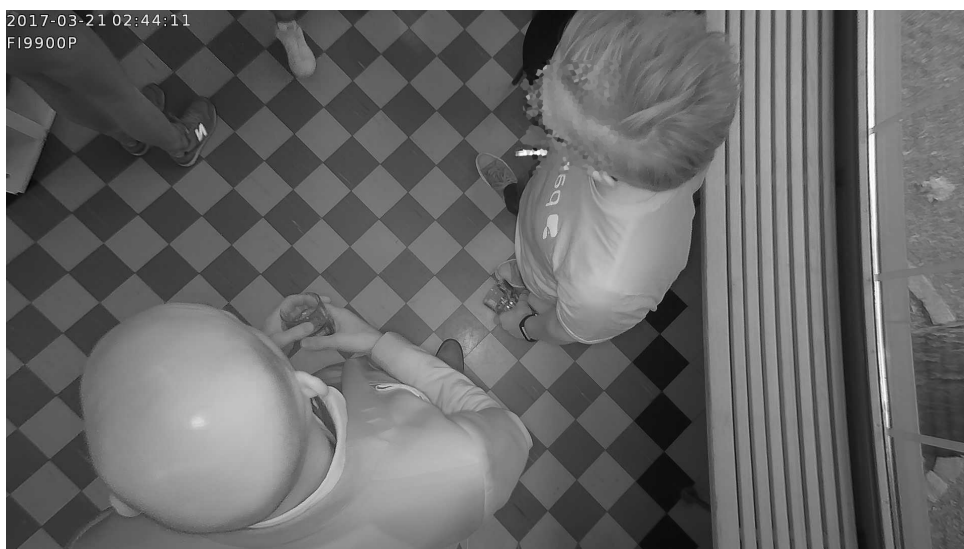
Figure 4.17: The IR-camera is at an orthogonal angle from the ceiling at Stena Center, which prevents the objects from covering each other at the same extent.
