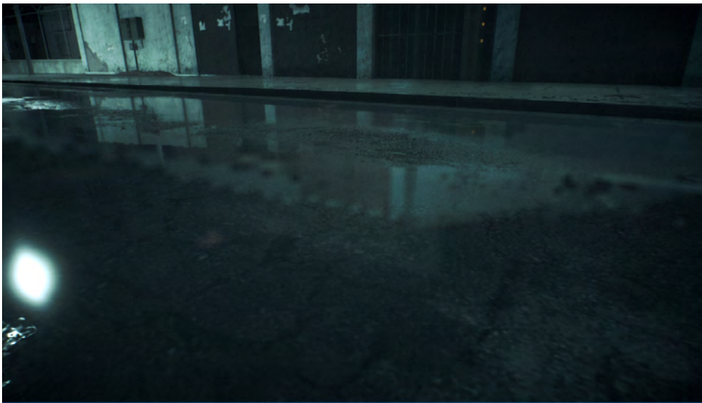
Figure 2.5: Lower resolution on cube maps are visible when compared with SSR.
