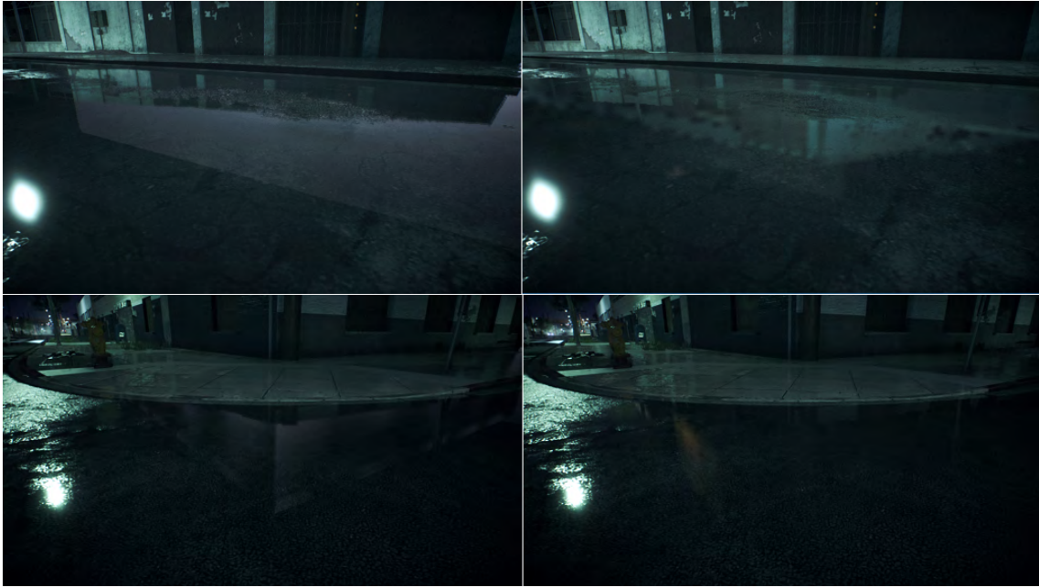
Figure 4.9: Images using proxy ray tracing (left column) and IBL cube maps (right column) to showcase how each implementation handles seaming screen space reflections together with off screen space reflections.
