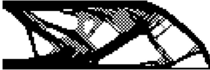
Figure 2.3: *The checkerboard problem shown on a simple finite element 2D geometry. Figure generated in MatLab with the topology optimization script [7].*
