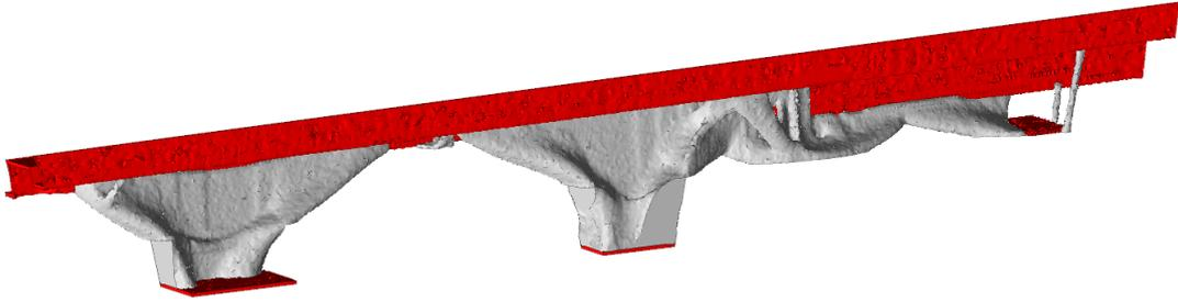
Figure 4.14: *Outside view of topology optimization results with additional support.*
