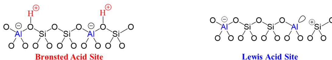
Figure 2.2: Brønsted and Lewis acid sites in zeolites. Adapted from Schulman et. Al. [2]
