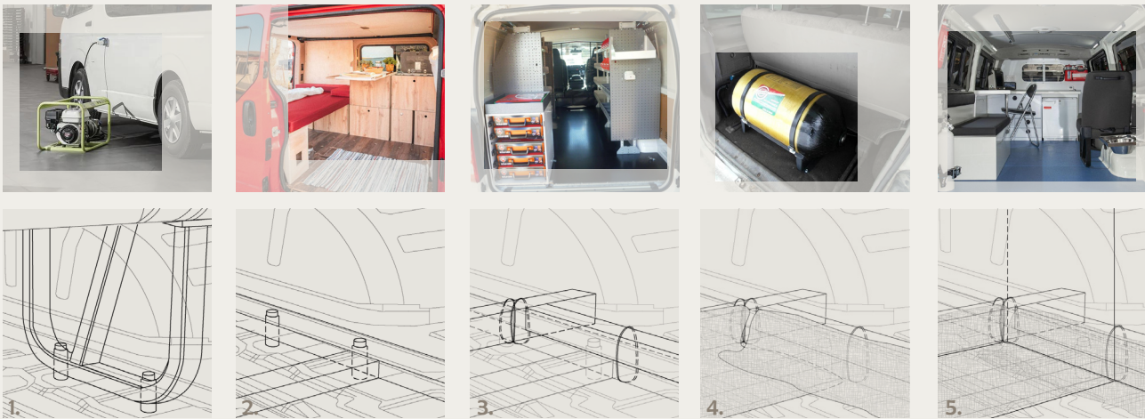
Figure 3.5.4. Modification of Toyota Hiace Picture Truck by author and Website from [Melusi, Pretoria]. Figure 3.5.5. Structural Installation Steps Drawn by author
