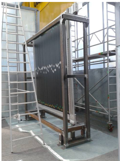
Figure 3.7: One of the NeuLAND double planes mounted with 100 bars. Behind the vertical bars 50 horizontal bars are mounted.
