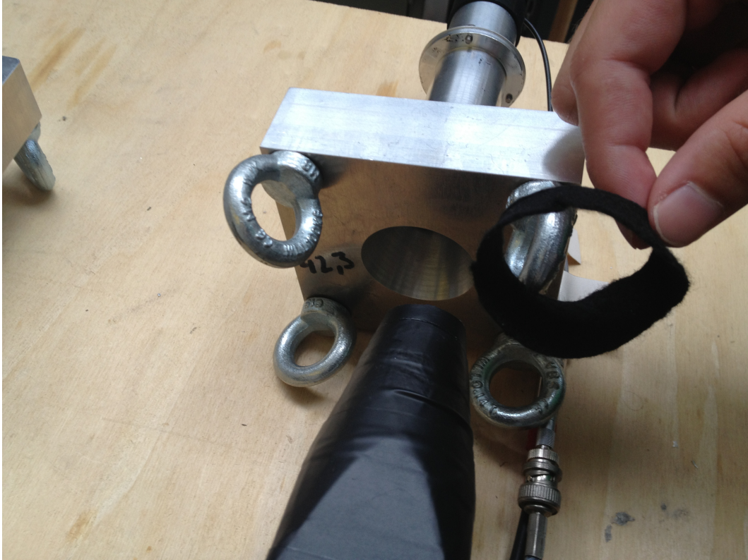
Figure 4.2: Bar together with the holder that goes on the light guide and a textile which is placed on the light guide to prevent environmental light from entering the PMT.
