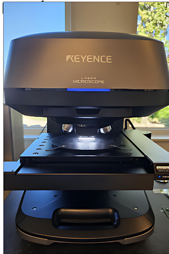
Figure 3.17: Keyence VK-3000 Laser Microscope.
