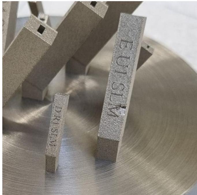
Figure 3.21: PBF-LB filter EU1 SLM.
