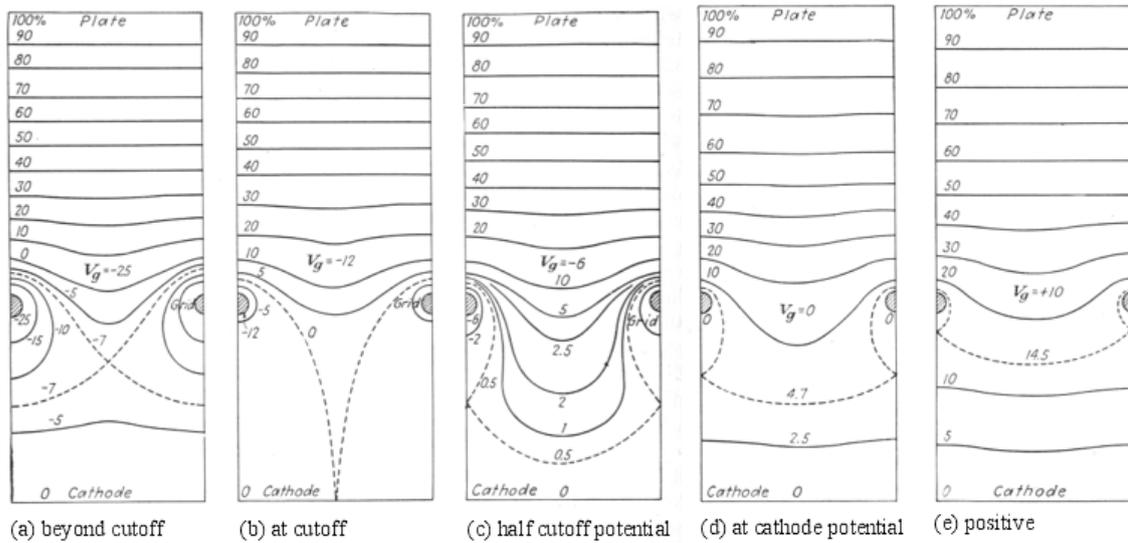
Figure 6: Electric field at several grid voltages (Harper, 2003)
