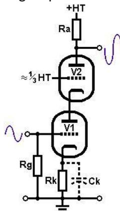
Figure 26: Cascode (Blencowe, The Cascode, 2011)
