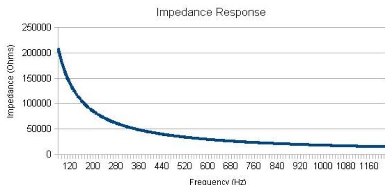
Figure 36: Impedance response of the attenuation circuit
