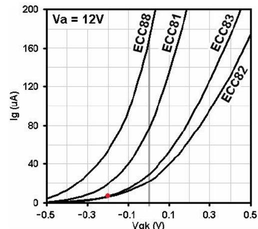
Figure 35: Grid current response of first gain stage
