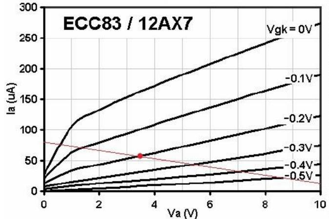
Figure 34: Load line analysis of the first triode stage
