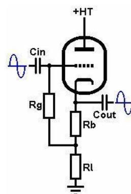
Figure 24: AC Coupled Cathode Follower (Blencowe, The AC-Coupled Cathode Follower, 2011)
