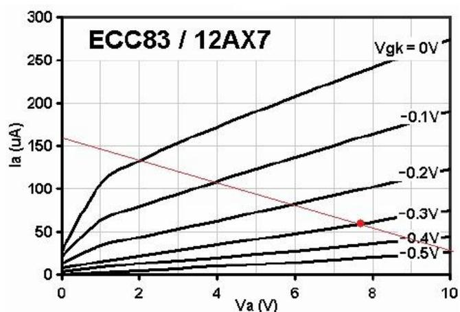
Figure 41: Load line analysis for redesigned second gain stage. A load-line for this anode resistance has been plotted in Figure 41. The original bias point has also
