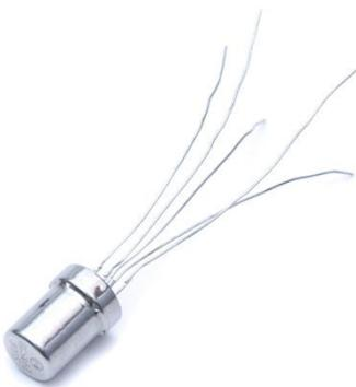
Figure 17: A vacuum tube nuvistor
