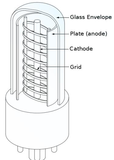
Figure 5: Section view of a vacuum tube triode
