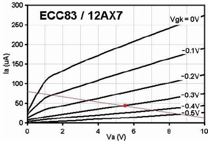
Figure 38: Load line analysis for second gain stage
