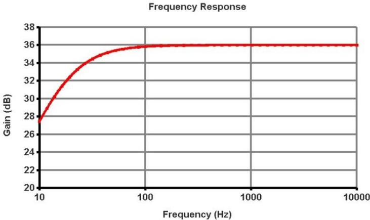
Figure 37: Frequency response of the circuit
