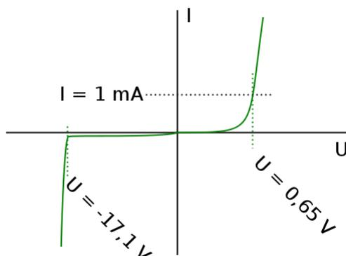
Figure 23: The behavior of a zener diode
