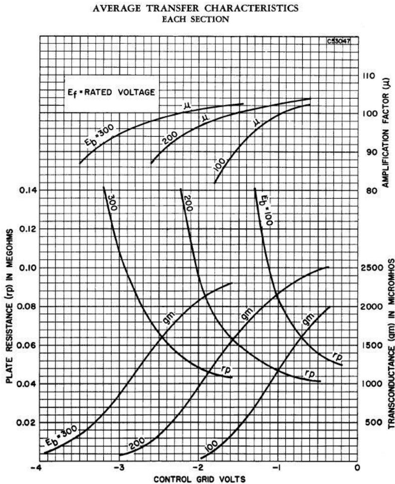
Figure 8: Effects of plate voltage on amplification factor (Sylvania Electronics Products Inc, 1955)
