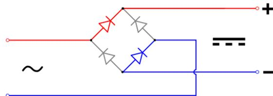
Figure 24: A schematic view of a diode bridge
