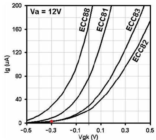
Figure 39: Grid voltage response of second stage
