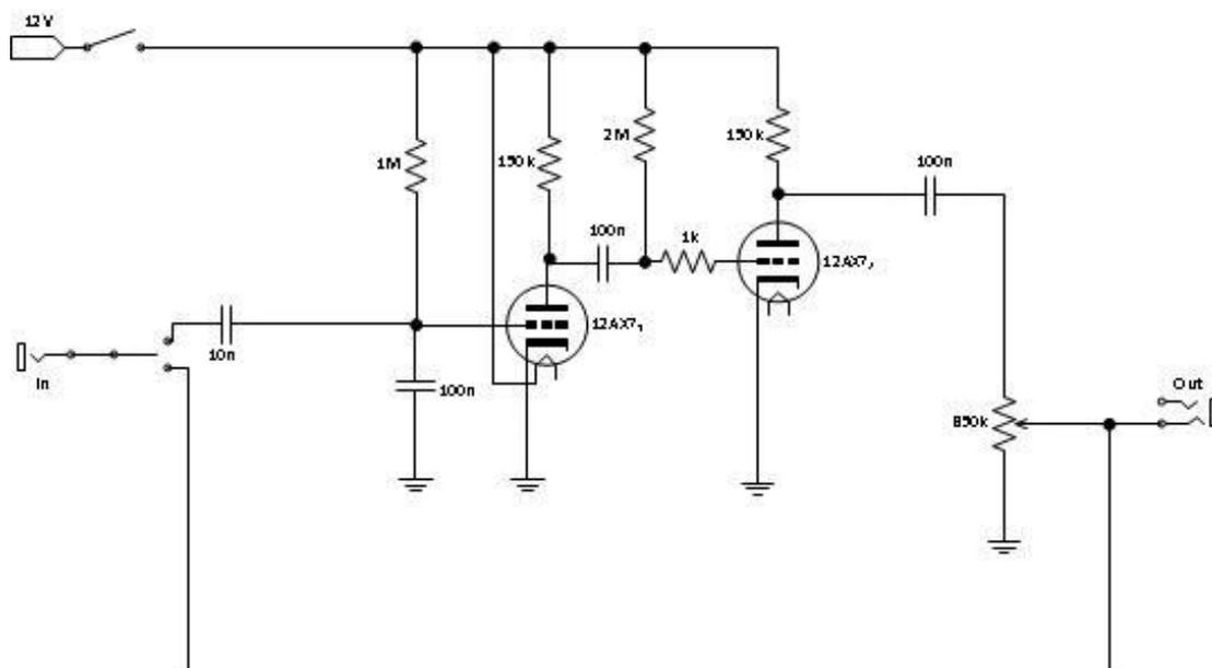
Figure 40: The initial circuit design
