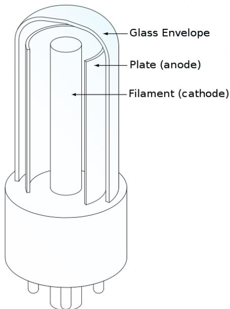
Figure 4: Section view of a vacuum tube diode
