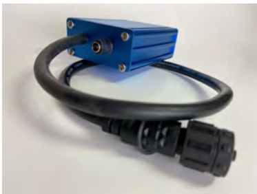
(a) The box containing a DMX to four-pin circuit.
