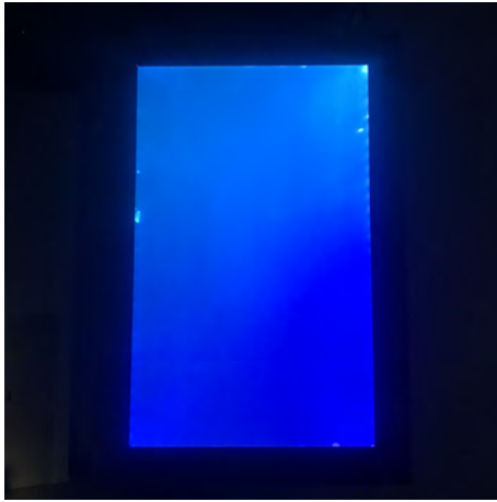
Figure 6.17: Bright areas appearing in in areas under pressure.
