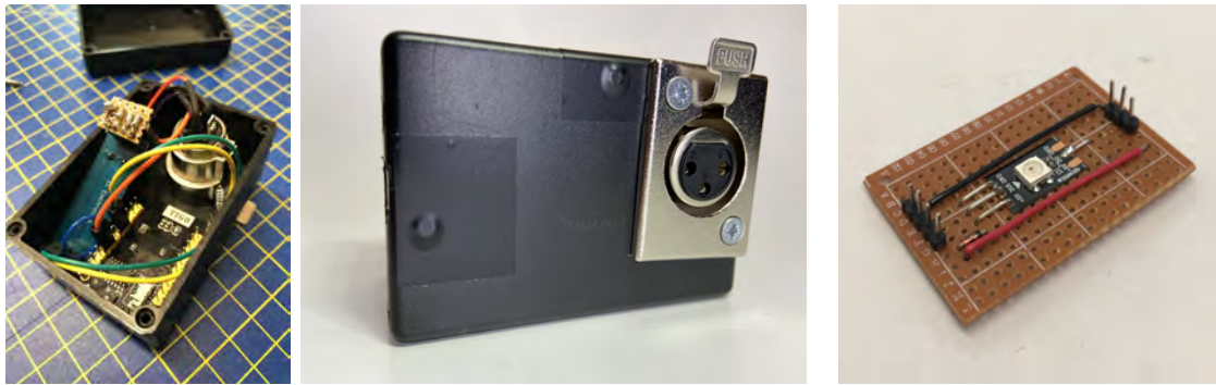
(a) Interior and exterior of the DMX to Wi-Fi node. (b) Sacrificial diode hack.
