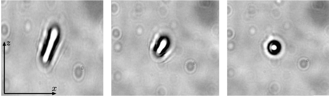
Figure 3.4: The figure shows the process of trapping a rod. The sequence from left to right, illustrates how the rod aligns with the direction of the laser, i.e. the beam axis, where it is in stable spatial equilibrium.
