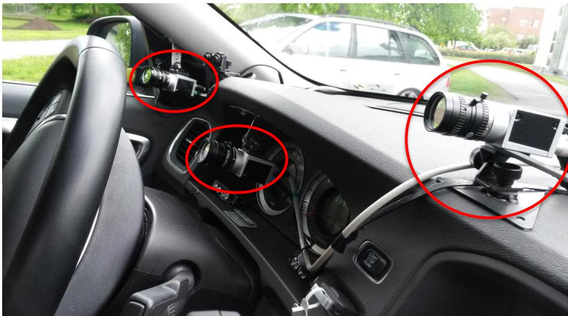
Figure 12: SmartEye set-up inside the passenger cabin
