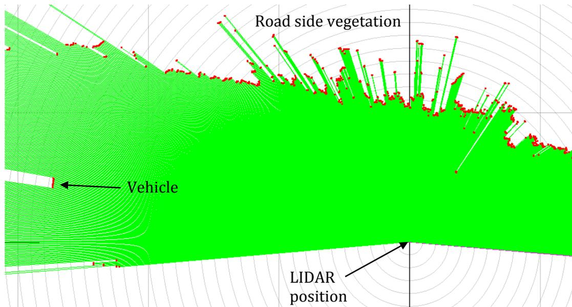
Figure 24: LIDAR data to identify phase one (red dots: spotted object; green area: no object spotted)
