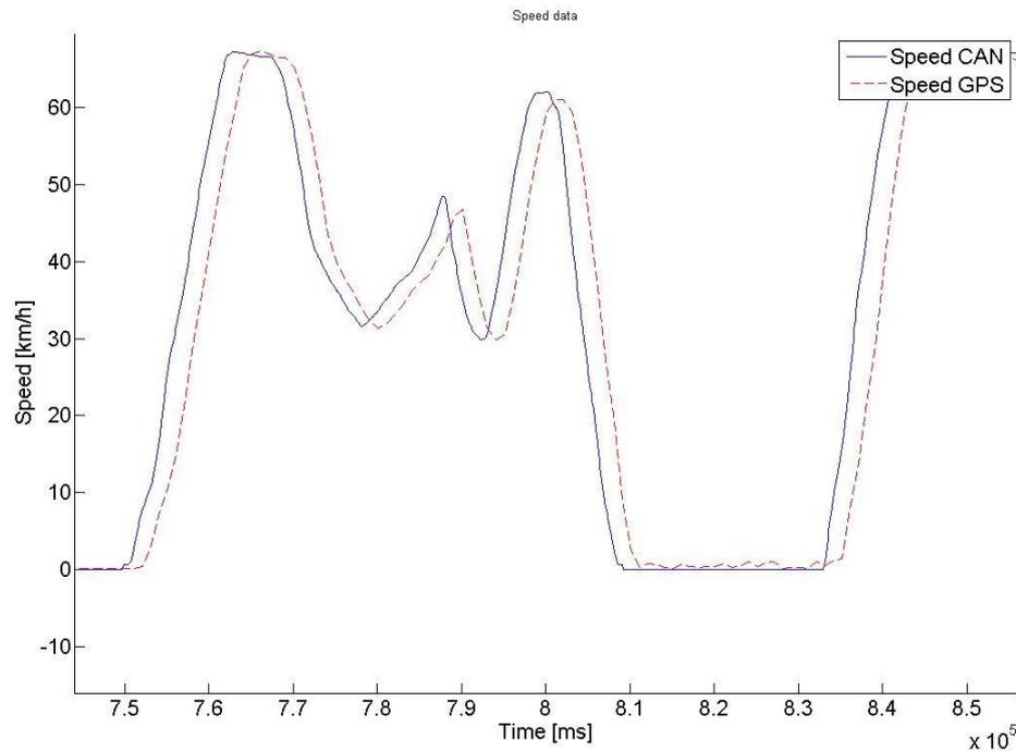
Figure 22: Compared speed data from CAN and GPS (raw data)
