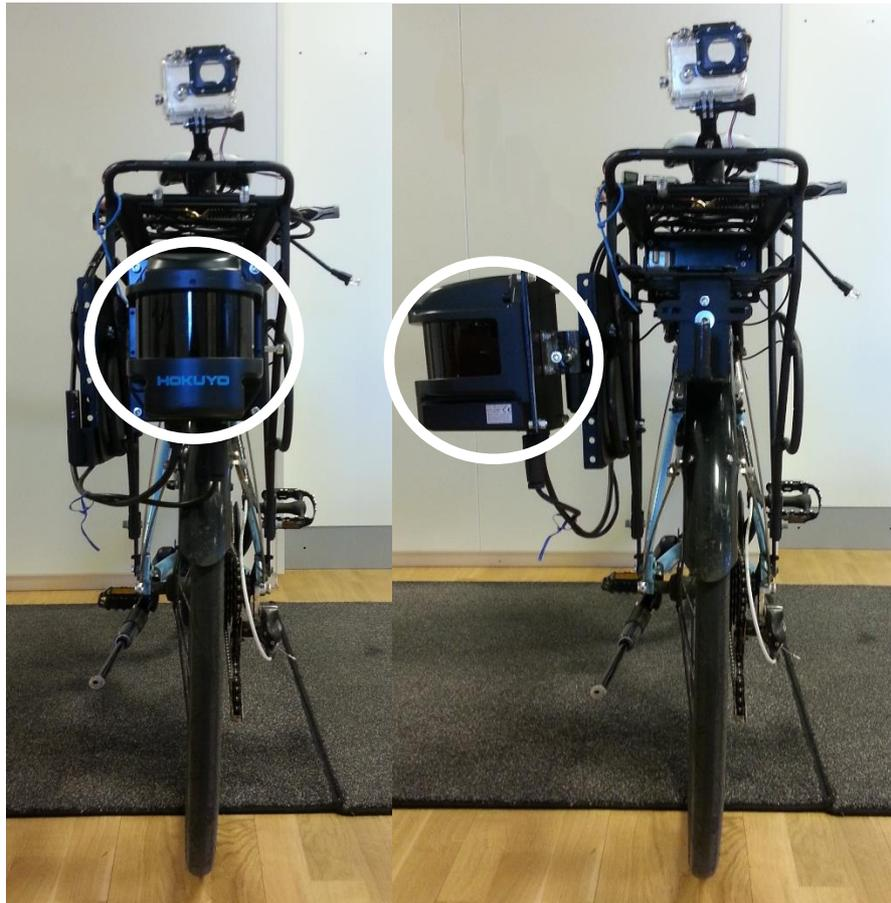
Figure 13: LIDAR mounting positions for pilot test
