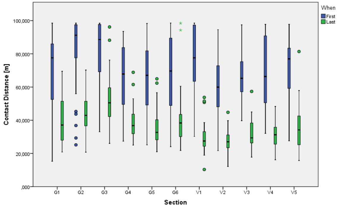
Figure 30: First and last contact distances of vehicles from the LIDAR
