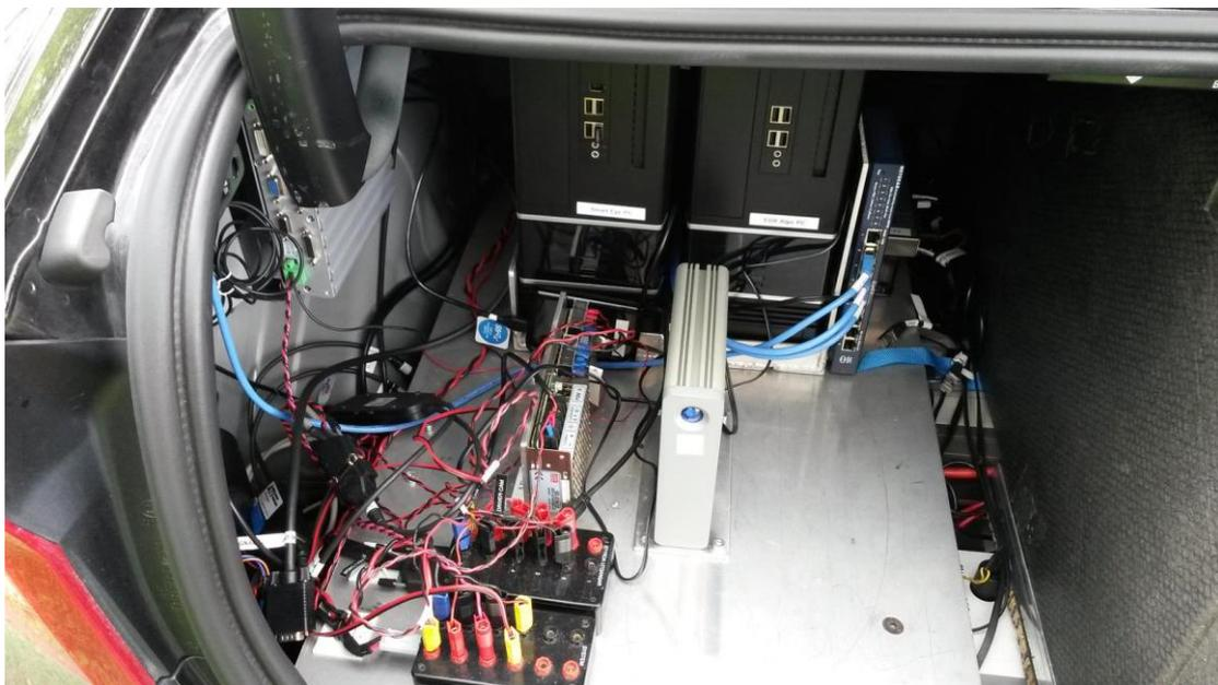
*Figure 11: CAN and SmartEye logger in the trunk of the car*
