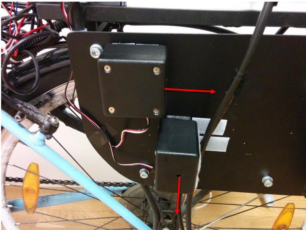
Figure 16: Mounting positions and directions of measurement of the pressure sensors
