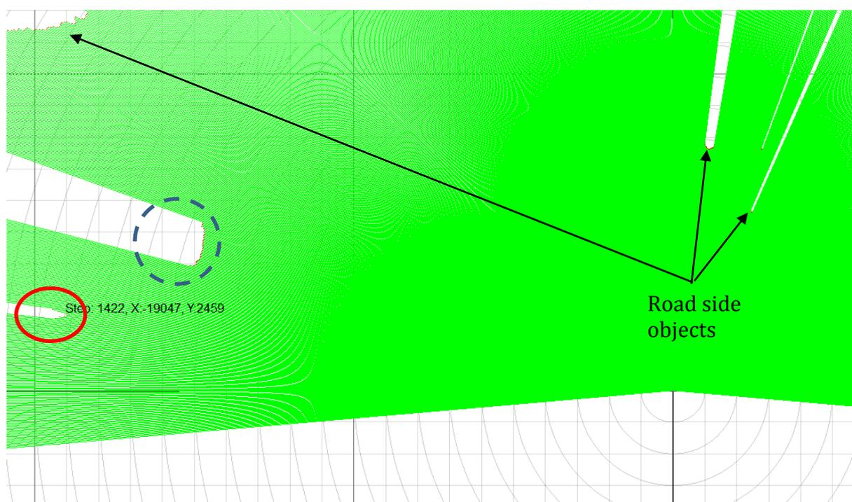
Figure 31: Bicycle and car in LIDAR data set (bicycle: red solid circle, car: blue broken circle)
