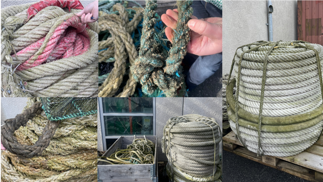
Figure 4.4: Worn-out mooring lines (Authors own pictures).
