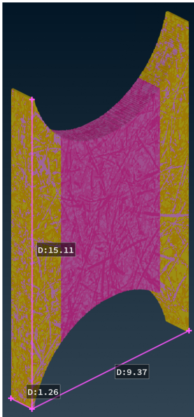
(a) KE1450. Dimensions: Height=15.11, Length=9.37, Thickness=1.26 (mm)
