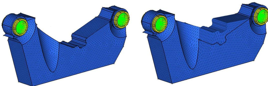
Figure 34 - Illustrates the shape limits of the top surface of the UCA in the shape and topology optimization.
