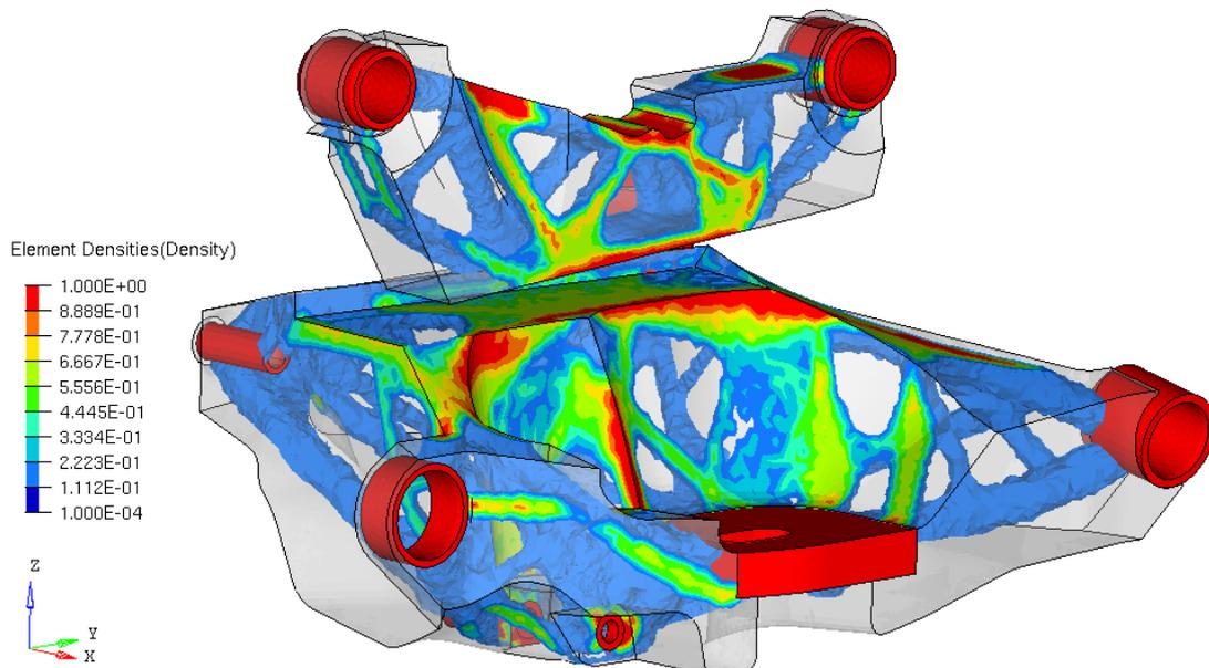
Figure 44 - Illustrates the obtained shape and topology optimization result from the combined model where shape change was allowed in the LCA's top and bottom surface and the UCA's bottom surface.
