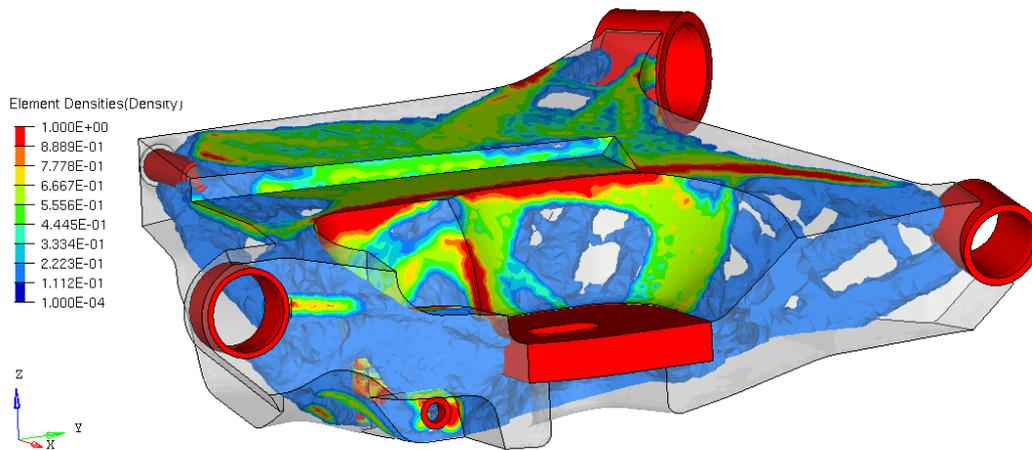
Figure 31 – Shows the topology optimization results of the LCA, used to identify high density regions.
