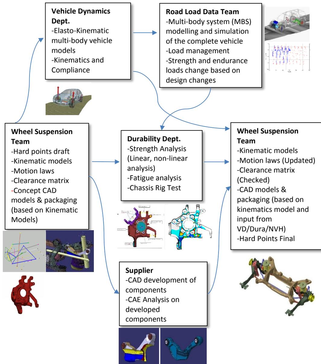
Figure 4 - Mapping of the current development process of components in the wheel suspension.
