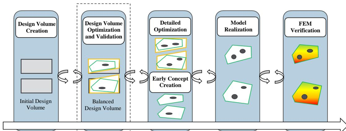
Figure 6 - Illustrates the proposed development process of components in the wheel suspension
