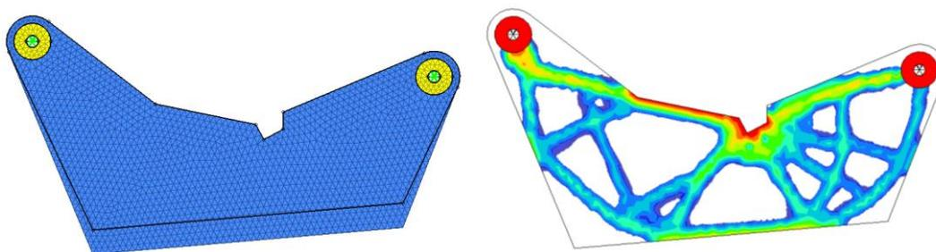
Figure 13 - Shows how the simplified UCA's bottom surface was morphed in negative Z-direction together with the result obtained from the topology optimization.
