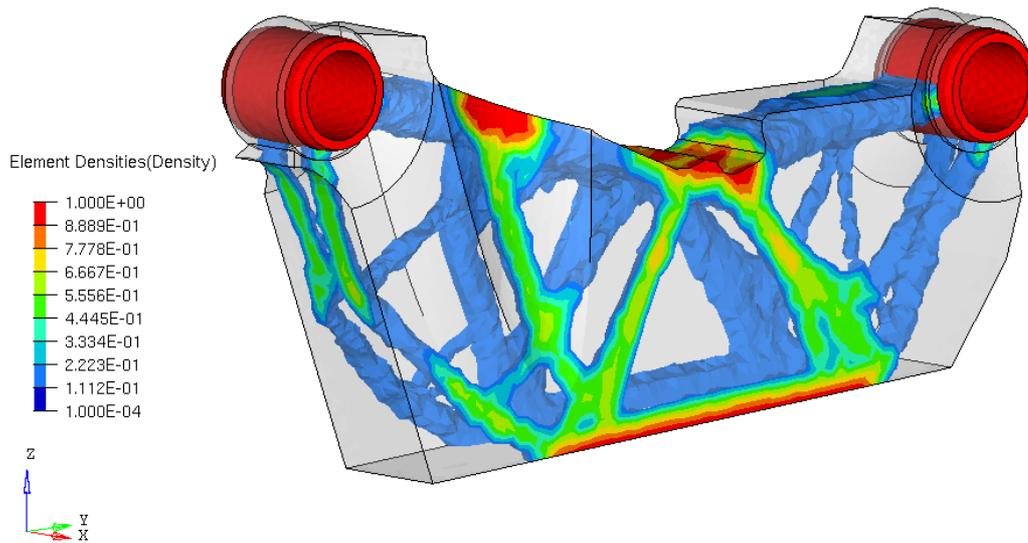
Figure 35 - Illustrates the obtained shape and topology optimization result when allowing shape change in the top surface of the UCA.
