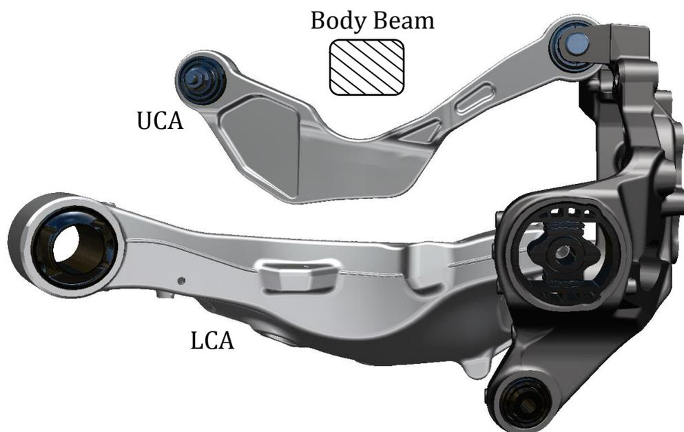
Figure 1 - Illustration of the conflict between the UCA and LCA
