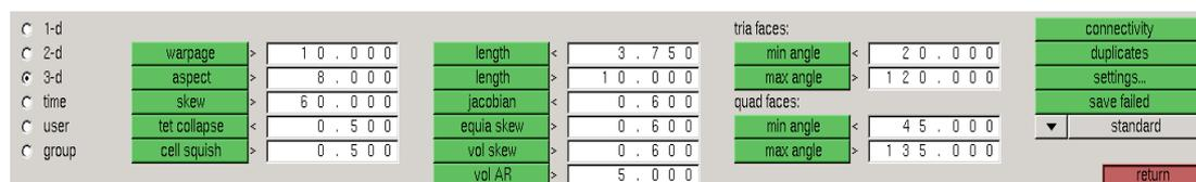
Figure 5 - Mesh checking panel
