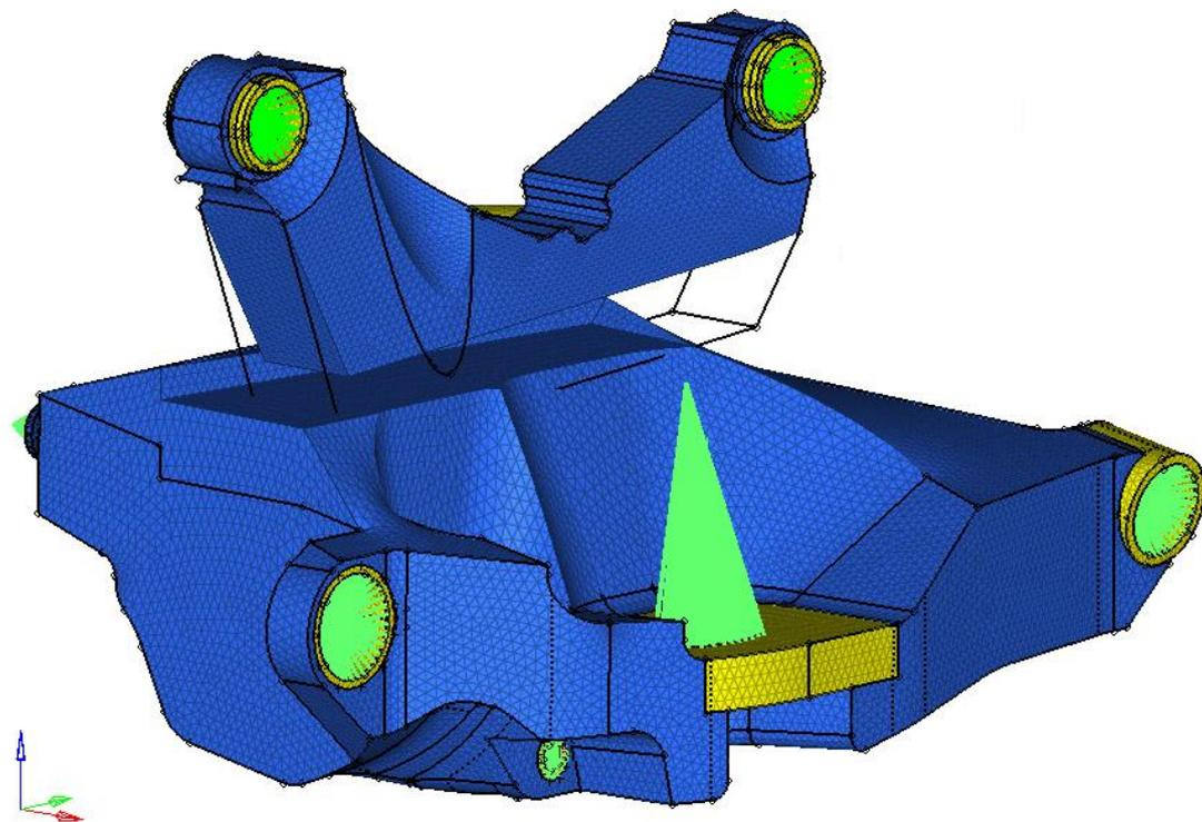
Figure 41 - Illustrates the shape limit in positive Z-direction of the combined bottom surface of the UCA and top surface of the LCA in the combined shape and topology optimization.
