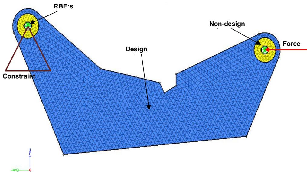
Figure 10 - Topology optimization settings of the simplified model of the UCA. The pictures shows how the models was split into design space and non-design space together with the RBE:s, constraint, and force that were applied to the model.
