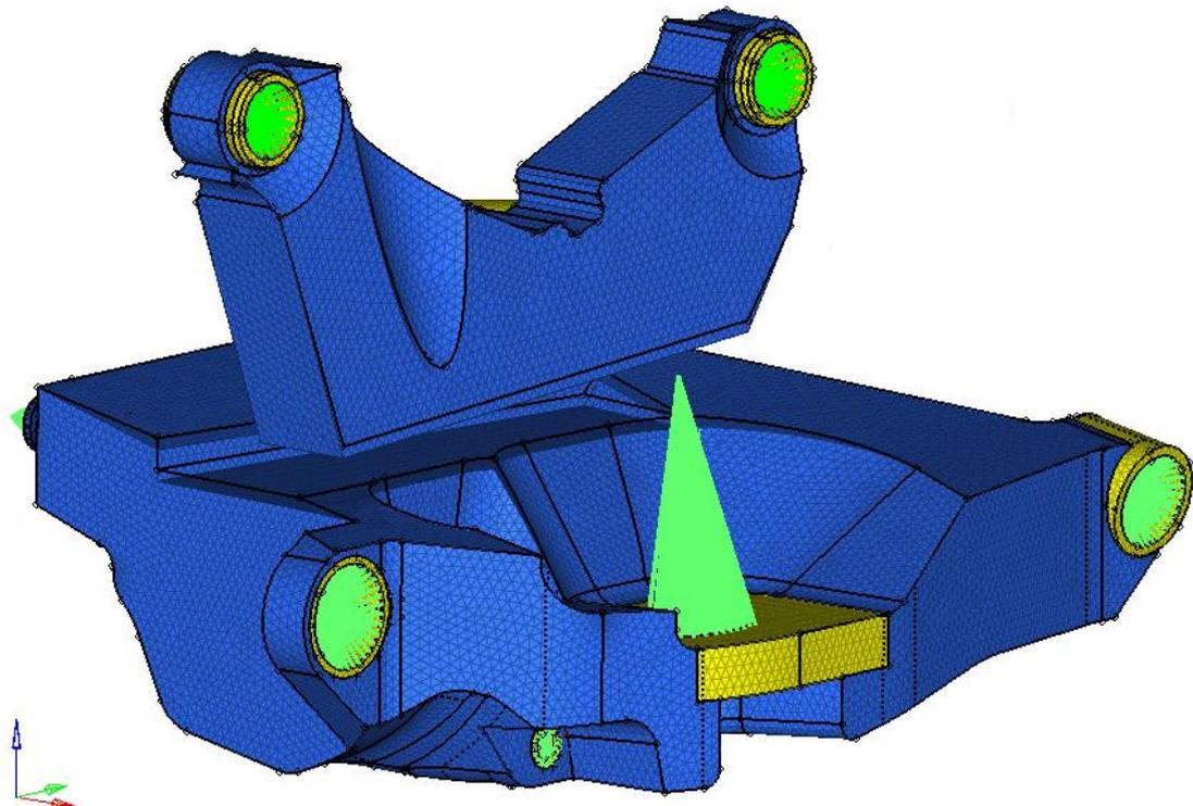
Figure 40 - Illustrates the shape limit in negative Z-direction of the combined bottom surface of the UCA and top surface of the LCA in the combined shape and topology optimization.
