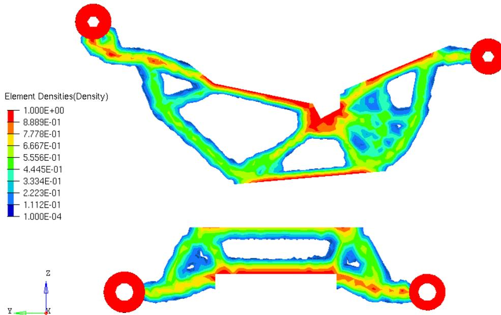
Figure 19 – Result obtained from the shape and topology optimization of the simplified combined model.
