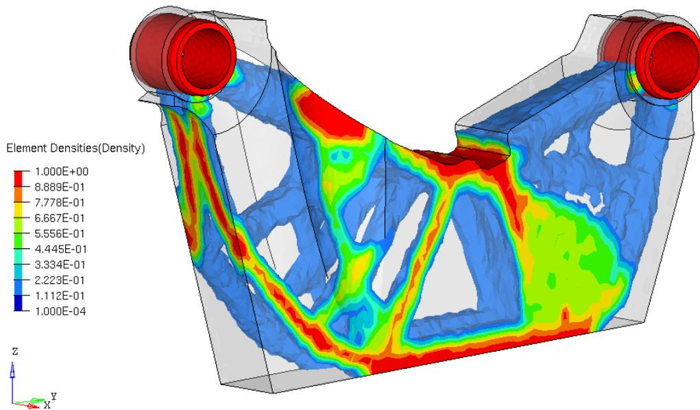
Figure 33 - Illustrates the obtained shape and topology optimization result when allowing shape change in the bottom surface of the UCA.
