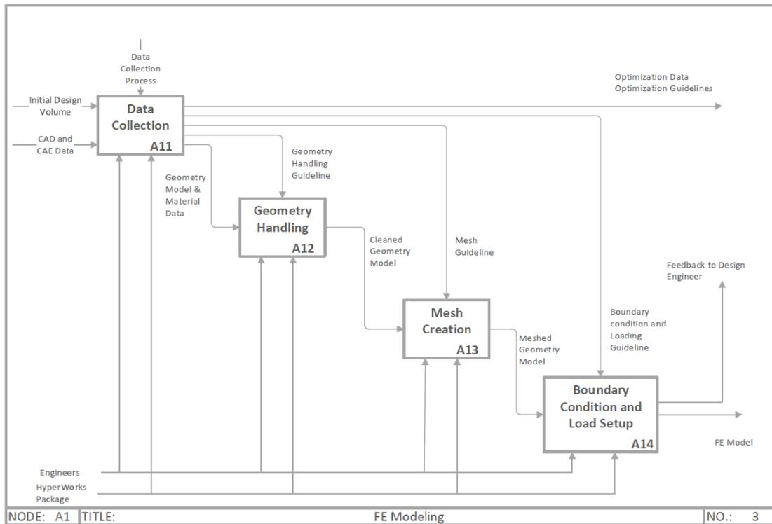
Figure 24 - Shows the third level of the IDEF0 diagram at node A1, illustrating the activities performed in the sub-function FE Modeling.
