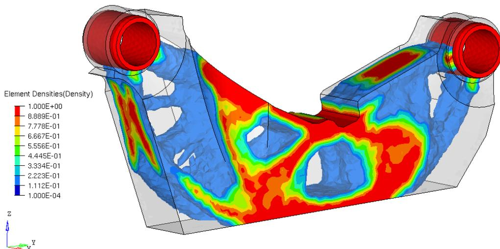
Figure 30 - Shows the topology optimization results of the UCA, used to identify high density regions.
