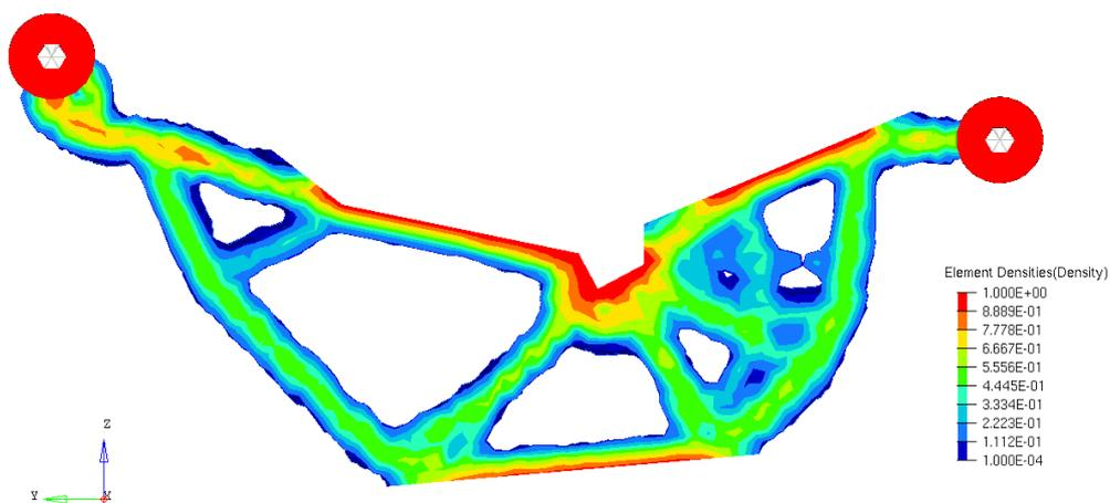
Figure 11 - Topology optimization result of the simplified UCA
