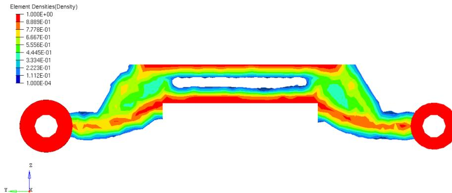
Figure 12 - Topology optimization result of the simplified LCA
