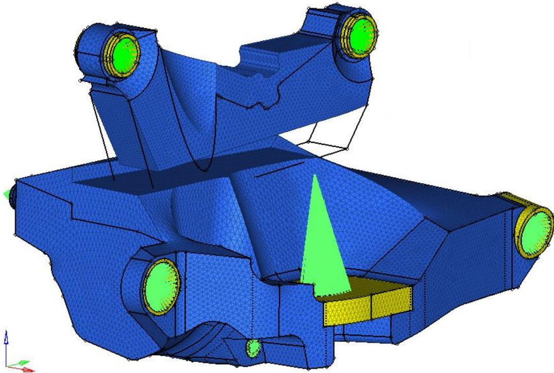
Figure 43 - Illustrates the shape limit of the combined bottom surface of the UCA and top surface of the LCA together with the limit of a second shape used on the top surface of the UCA.
