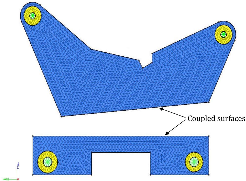
Figure 17 – Illustration of the coupled surfaces in the simplified combined model, used in the shape and topology optimization
