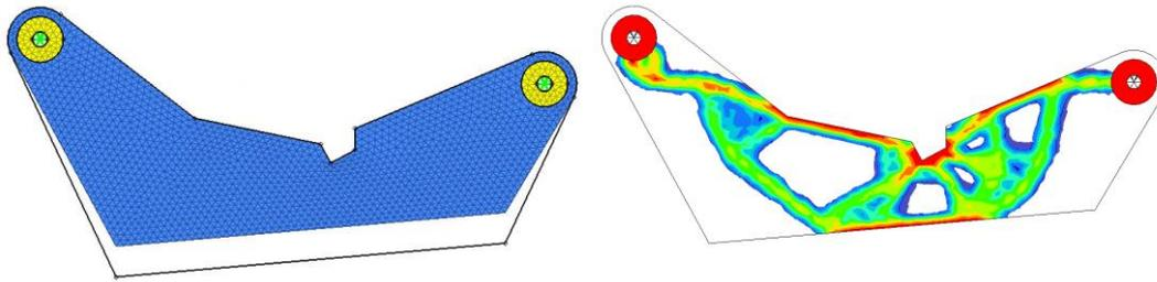
Figure 14 - Shows how the simplified UCA's bottom surface was morphed in positive Z-direction together with the result obtained from the topology optimization.
