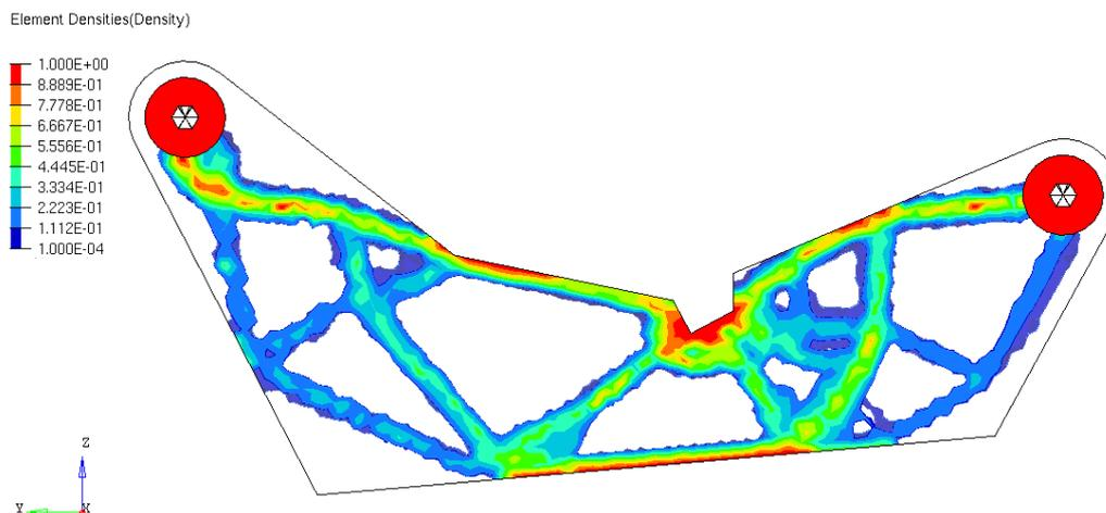
Figure 21 - Result obtained from the shape and topology optimization of the UCA with a MINDIM value of 5.
