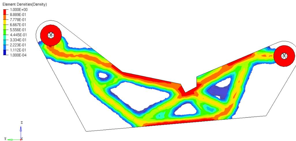
Figure 20 - Result obtained from the shape and topology optimization of the UCA with a MINDIM value of 30.
