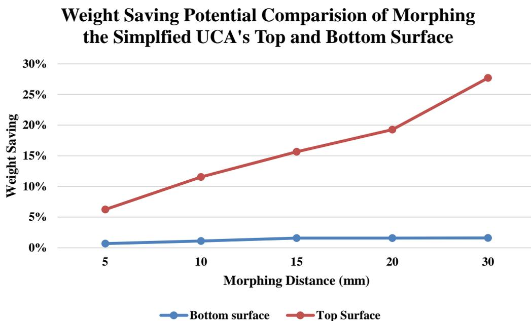
Figure 16 - Graphical representation of the weight saved from bottom and top surface morphing
