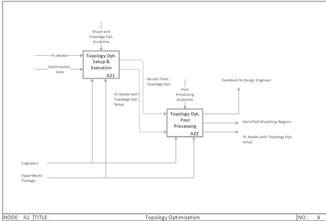
Figure 25 - Shows the third level of the IDEF0 diagram at node A2, illustrating the activities performed in the sub-function Topology Optimization.
