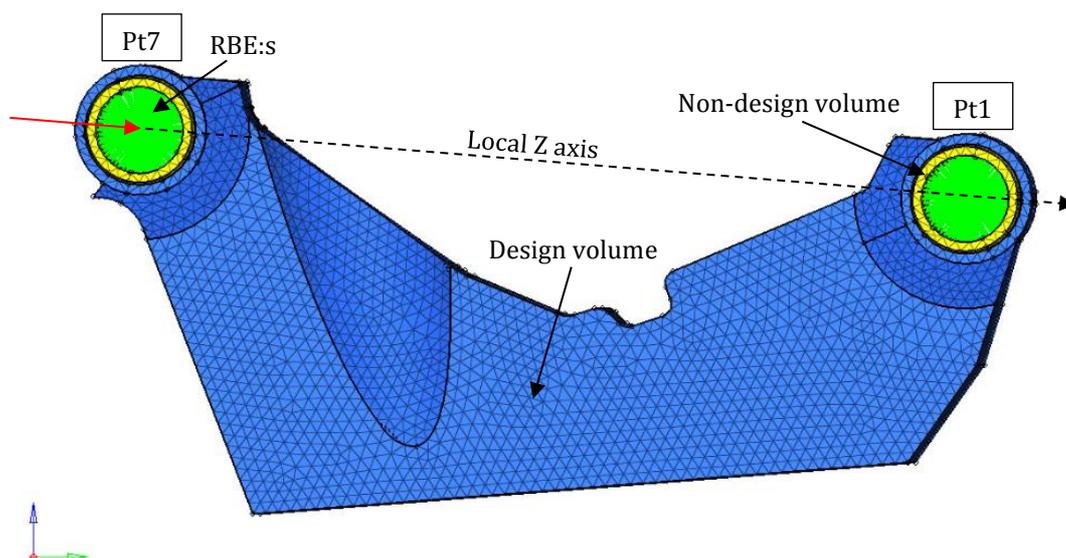
Figure 28 - Shows the model setup to the UCA.
