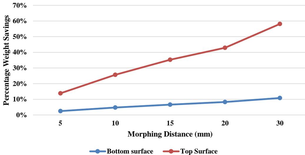
Figure 36 - Graphically illustrates the weight saving potential when morphing the top compared to the bottom surface of the UCA.
