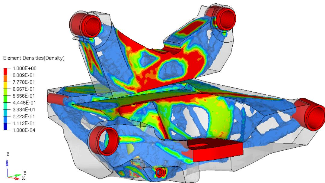
*Figure 42 - Illustrates the obtained shape and topology optimization result from the combined model where shape change was allowed in the LCA's top surface and the UCA's bottom surface.*
