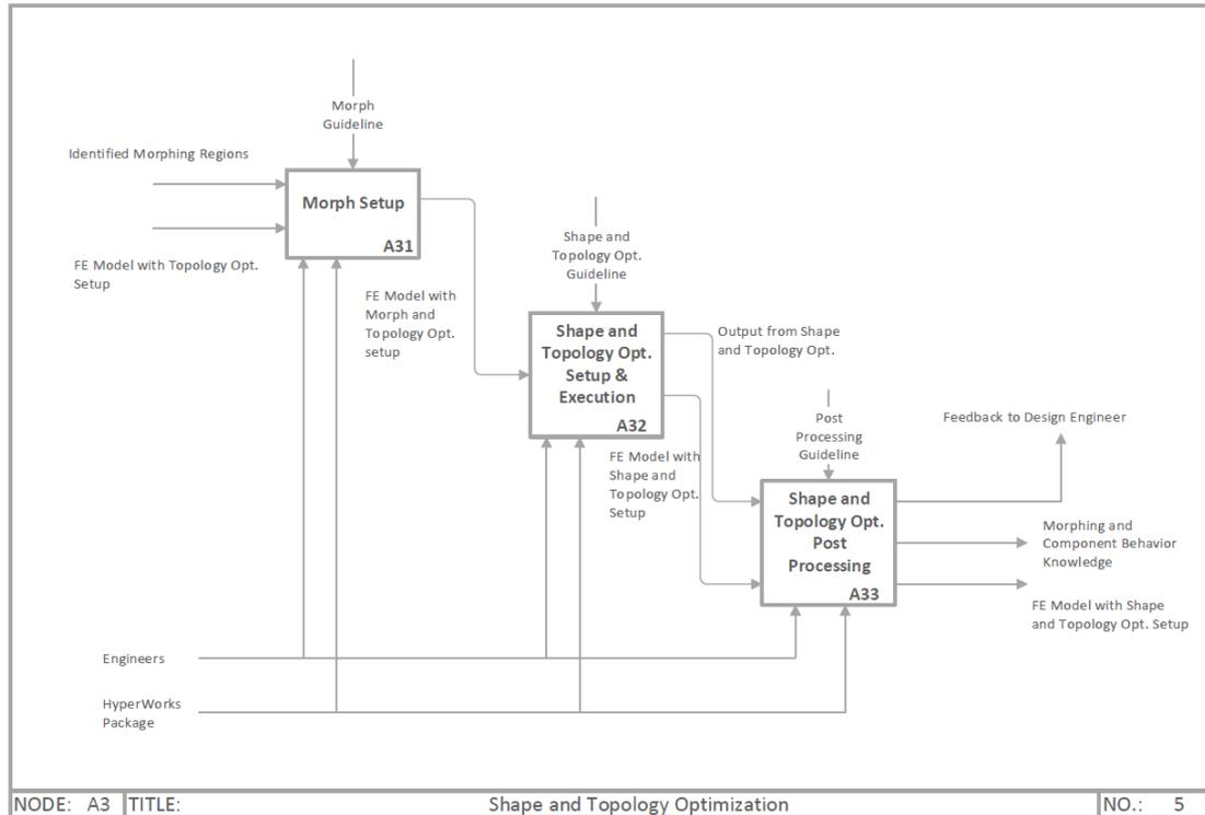
Figure 26 - Shows the third level of the IDEF0 diagram at node A3, illustrating the activities performed in the sub-function Shape and Topology Optimization.
