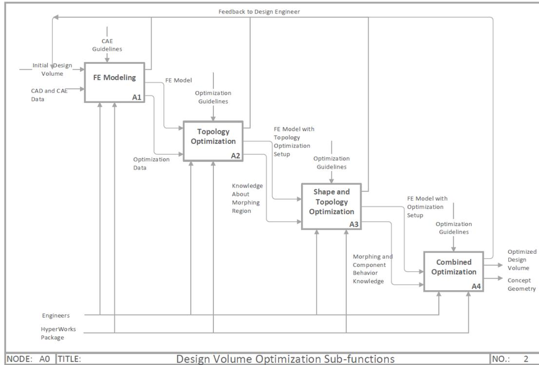
Figure 23 - Shows the second level of the node A0 in the IDEF0 diagram, illustrating the four sub-functions of the process; FE Modeling, Topology Optimization, Shape and Topology Optimization, and Combined optimization.
