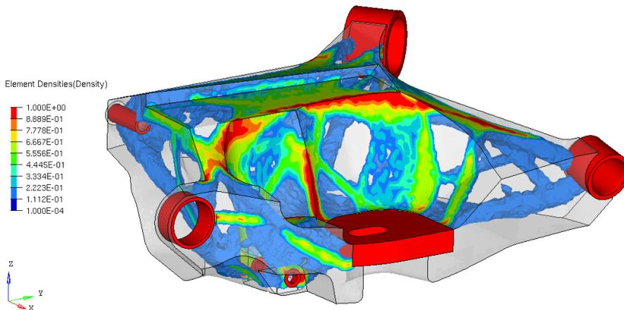
Figure 39 - Illustrates the obtained shape and topology optimization result when allowing shape change in the top surface of the LCA.
