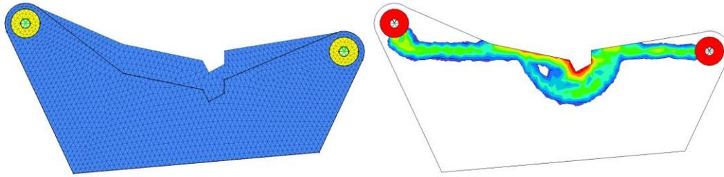
Figure 15 - Shows how the simplified UCA's top surface was morphed in positive Z-direction together with the result obtained from the topology optimization
