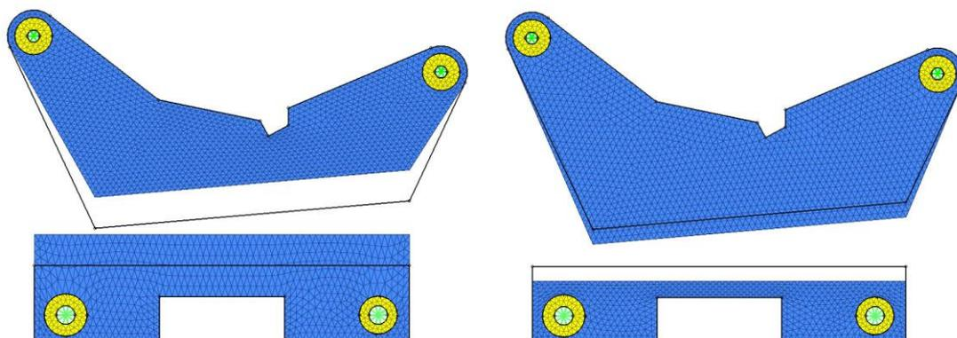
Figure 18 - Illustrates how the simplified combined model was morphed in positive and negative Z-direction
