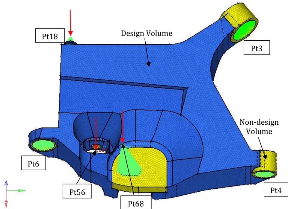
Figure 29 – Shows the model setup of the LCA.
