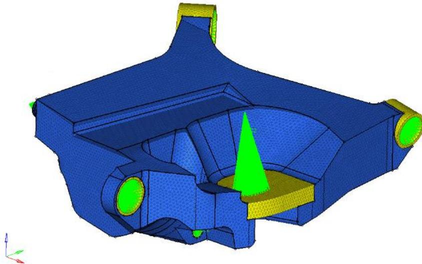
Figure 37 - Illustrates the shape limit in negative Z-direction of the top surface of the LCA in the shape and topology optimization.
