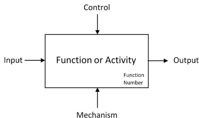
Figure 3 – Illustrates the basic structure of an IDEF0 diagram
