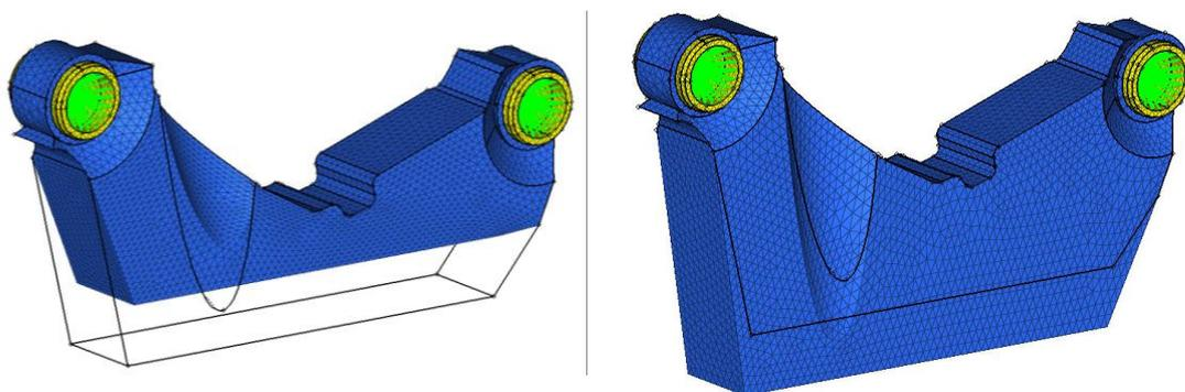
Figure 32 - Illustrates the shape limits of the bottom surface of the UCA in the shape and topology optimization.
