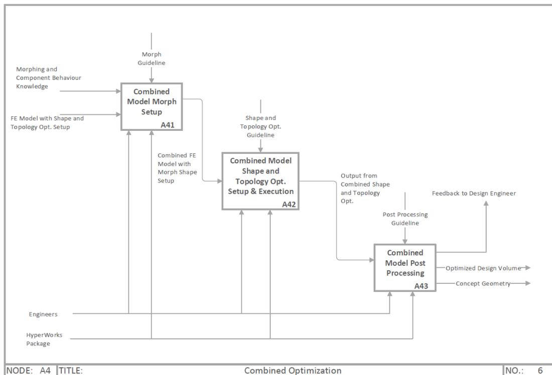
Figure 27 - Shows the third level of the IDEF0 diagram at node A4, illustrating the activities performed in the sub-function Combined Optimization.
