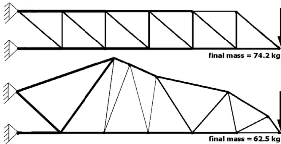
Figure 2 - Illustrates the change in topology design by varying the design space [25]
