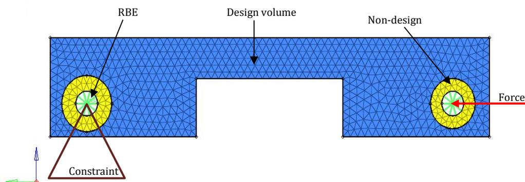
Figure 9 - Topology optimization settings of the simplified model of the LCA. The picture shows how the model was split into design space and non-design space together with the RBE:s, constraint, and force that were applied to the model.
