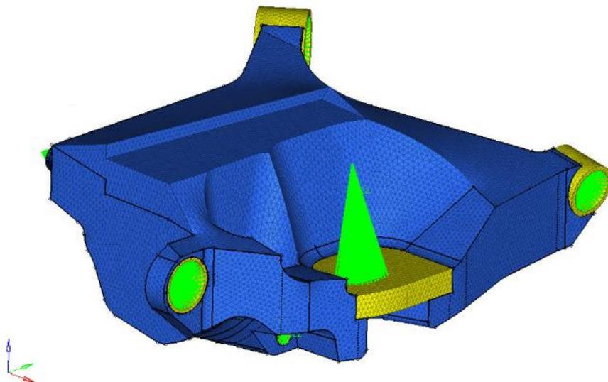
Figure 38 - Illustrates the shape limit in positive Z-direction of the top surface of the LCA in the shape and topology optimization.
