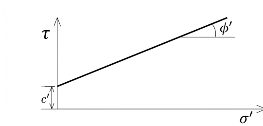
Figure 6.1: Mohr-Coulomb failure envelope
