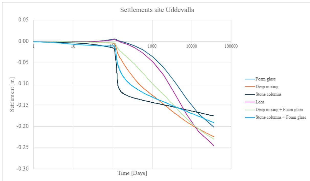
Figure 8.12: Settlement over time for the different ground improvement techniques at the Uddevalla site
