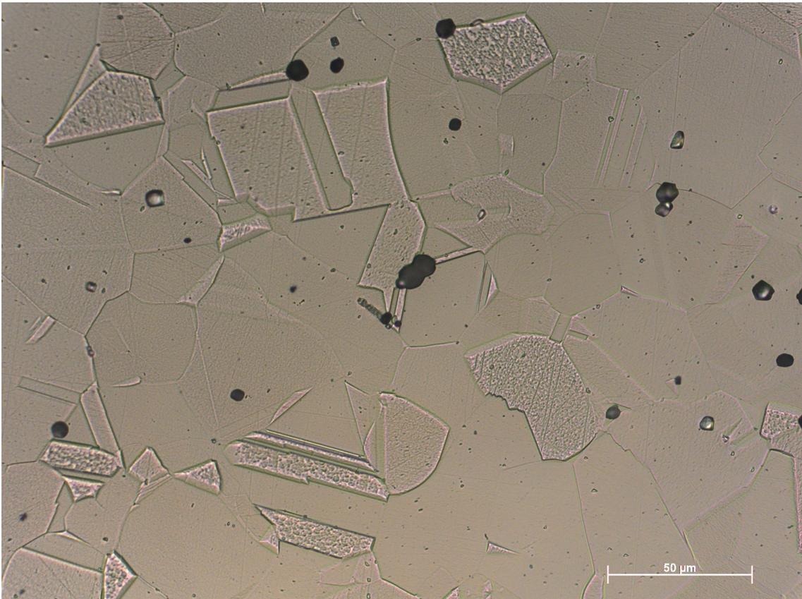
**Figure A.4:** Microscopy image showing microstructure of a 316L sample from *Supplier B*, captured on *Sample 2* from a random spot within the radial depth of 16,0 – 19,5mm.
