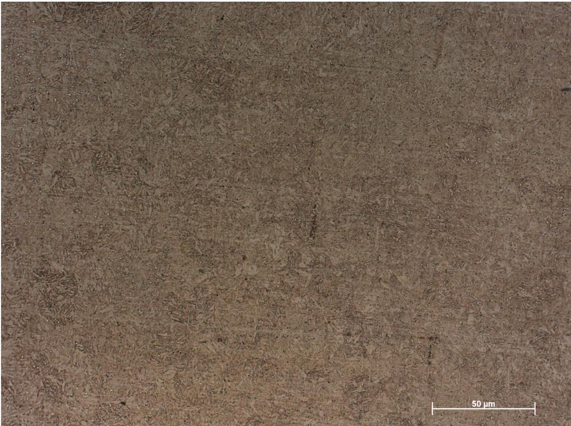
**Figure B.3:** Microstructure of 100Cr6 in *Hardening 2* condition.
