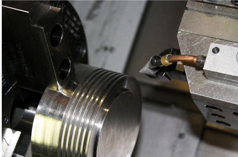
**Figure 3.8:** The figure illustrates the experimental setup for the face turning of the 316L workpieces without the nose engaged. Note that the insert is censored.
