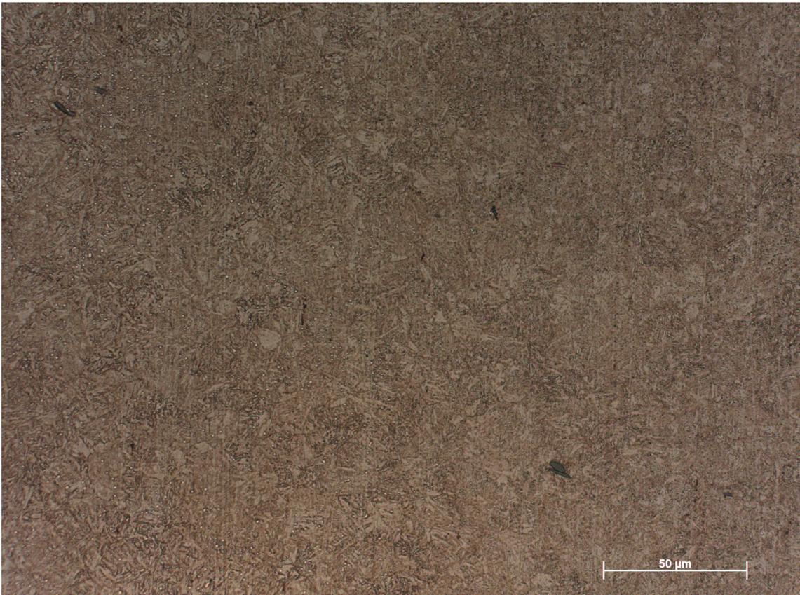
**Figure B.2:** Microstructure of 100Cr6 in *Hardening 1* condition.
