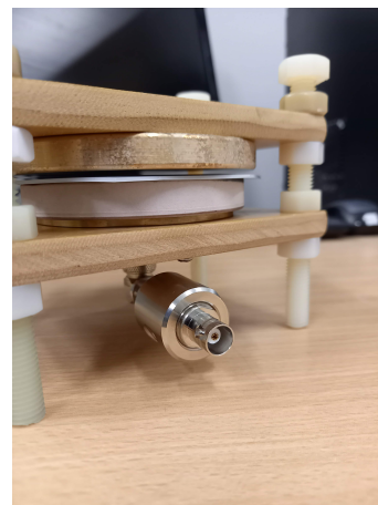
(b) Electrode arrangement for loss factor measurement with silicon rubber sample.
