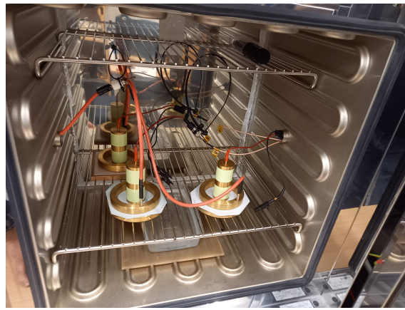
Figure 3.16: Surface resistivity measurement arrangement.
