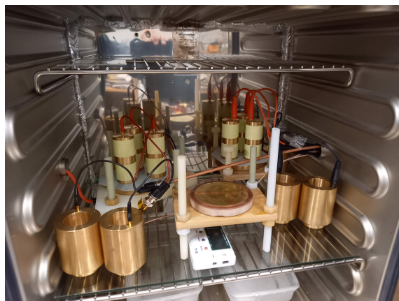
(b) Bulk resistivity measurement arrangement without guards.
