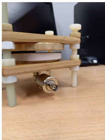
(a) Electrode arrangement for loss factor measurement without silicon rubber sample.
