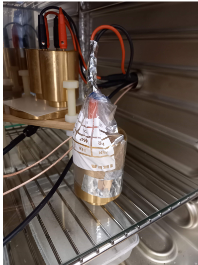
Figure 4.5: Plastic bag to protect the electrodes from water condensation.
