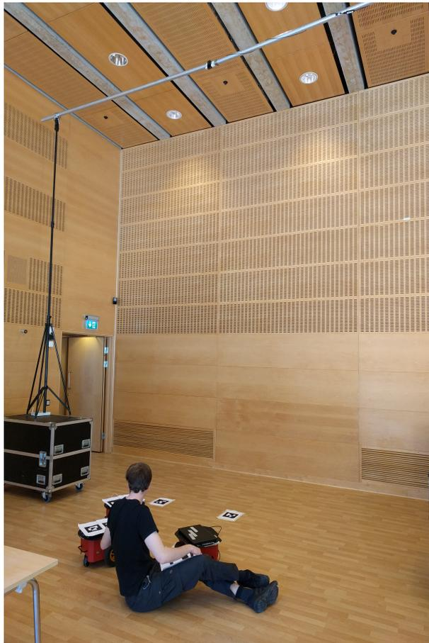
**Figure 4.4:** Overview of the camera tracking system. The camera is mounted on an aluminium pipe suspended between two tripods standing upon two cases. The estimated height of the camera is  $\approx 5.3$  m.
