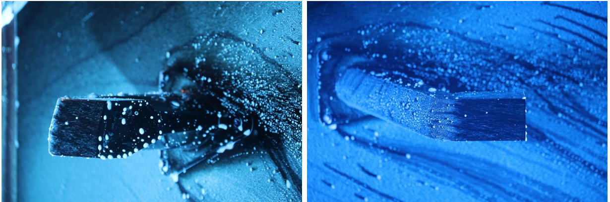
Figure 4.14: Rear and front view of final baseline CMS contamination by water droplets at 70 km/h, retrieved from the Wedgeoid experiment in the wind tunnel.
