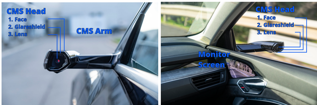
Figure 1.2: Exterior view of CMS (L) [7] and interior view of CMS and monitor (R) [8], belonging to an Audi e-tron. Parts of interest are marked.
