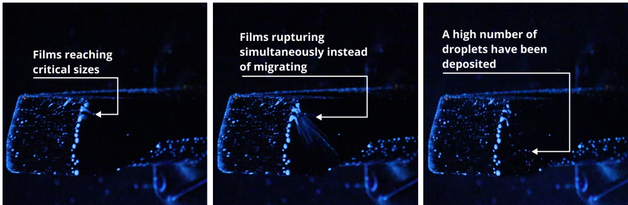
Figure B.9: Example of when film rupture is favored over droplet migration, on baseline CMS in 120 km/h from Wedgeoid experiment.
