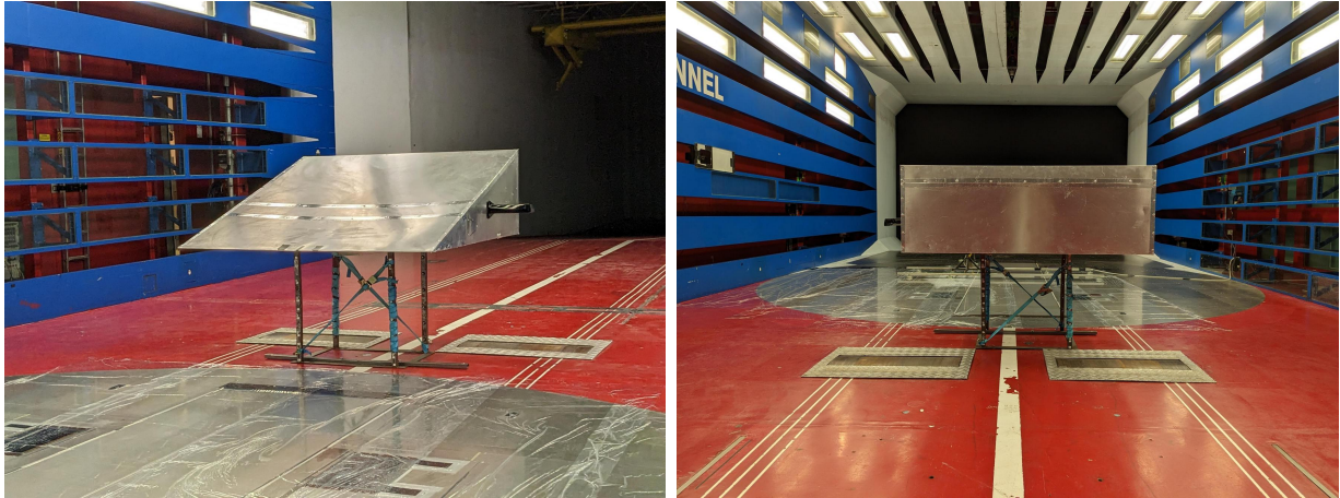
Figure A.2: Base setup of Wedge with attached CMS in the wind tunnel.
