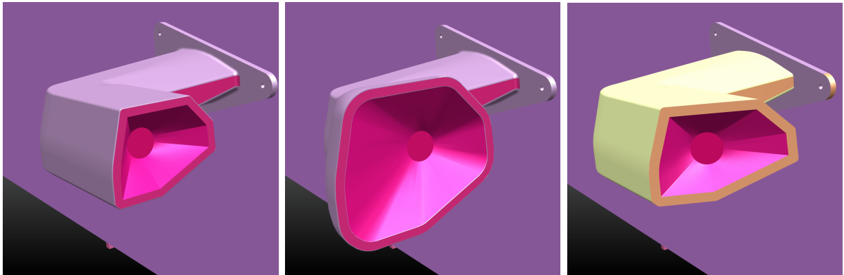
Figure 3.3: View of Deeper (L), Enlarged (M) and Slanted GS designs (R).
