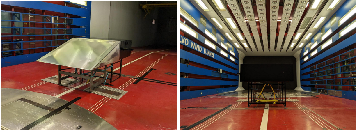
Figure 3.7: Views of Wedgeoid with attached baseline CMS in wind tunnel.
