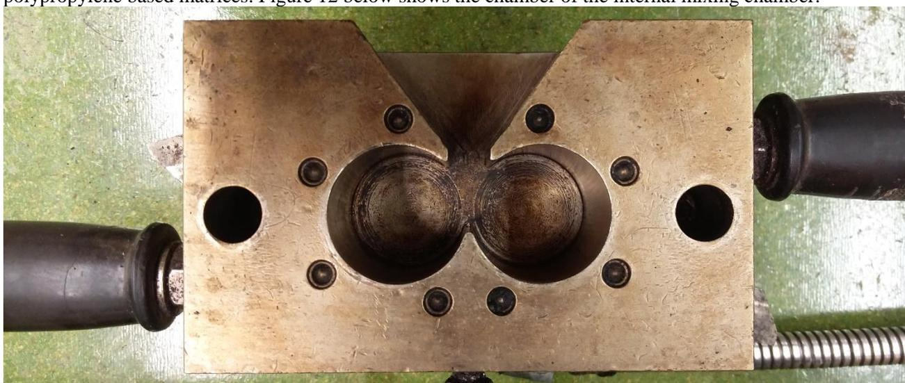
Figure 12, Internal mixing chamber of compounder.
