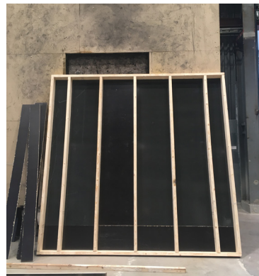
Panel made with pinewood and temporary back shuttering for casting.
