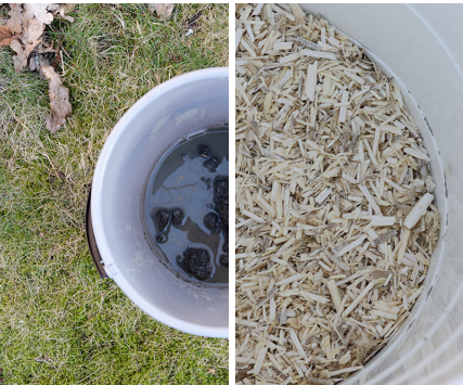
Preparation of clay and water in one bucket, hemp shivs in another bucket.
