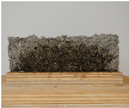
After 3 days, the corners are dried out. The surface while drying is quite fragile and brittle. Pieces can come of if handled without care.
