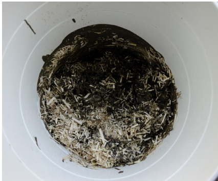
Mixing the shiv and clay-slip thoroughly, all the shiv must be coated with slip and a homogenous mix is to be prepared.
