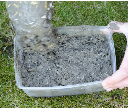
Mold the hemp-clay into a form. The sample can be demolded immediatly and left to dry.
