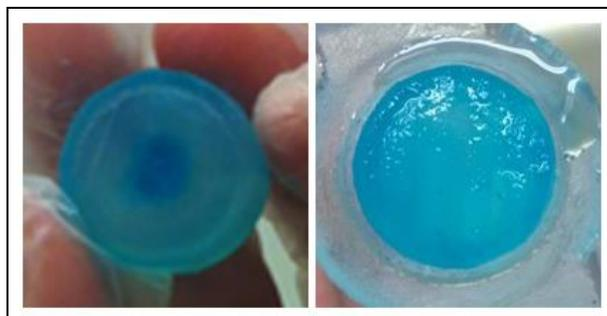
**Figure 34:** Alginate after flow through tests; Rectangular design (left) and conical design (right)
