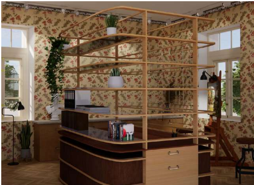
Image 52. Perspective: Room 109, with the addition of multifunctional furniture, that can be used for storage, bookshelves, working space for one conservator, and hanging grid for notes. The furniture has been placed in the center to achieve circulation in the room and preserve the walls in their current condition.
