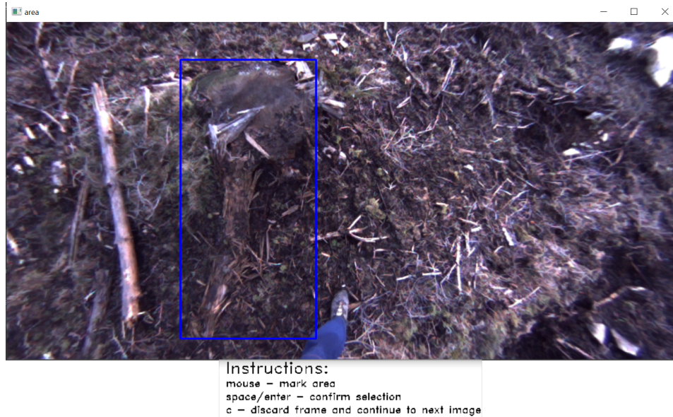
Figure 3.6: Example of how the custom GUI is used to isolate certain areas in the data. All images in the data set are displayed in series. If the user manually selects a region of interest, i.e. a stump, the selected area will be reshaped to fit the model requirements and then passed on to the mask creating tool seen in Figure 3.7. A list of instructions can be seen at the bottom of the image, displaying all possible actions.
