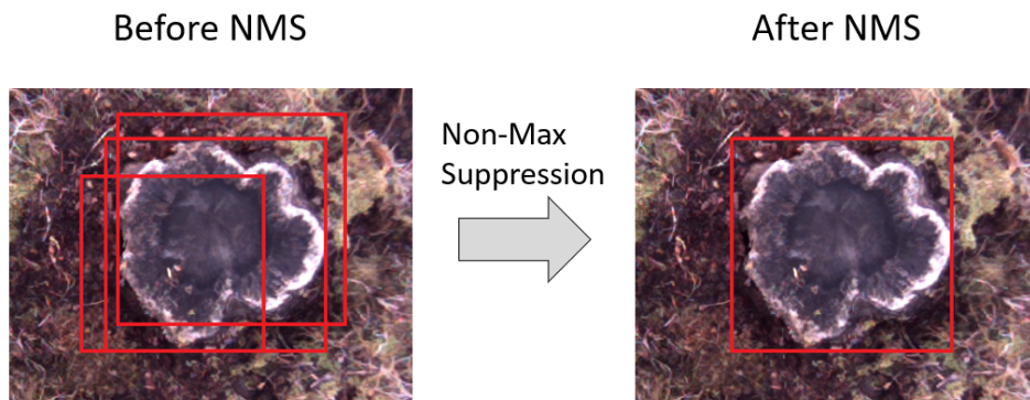
Figure 2.8: Proposed bounding boxes before (left) and after (right) non-maximum suppression is applied. Only the box with the highest accuracy score is kept, while the others are discarded.
