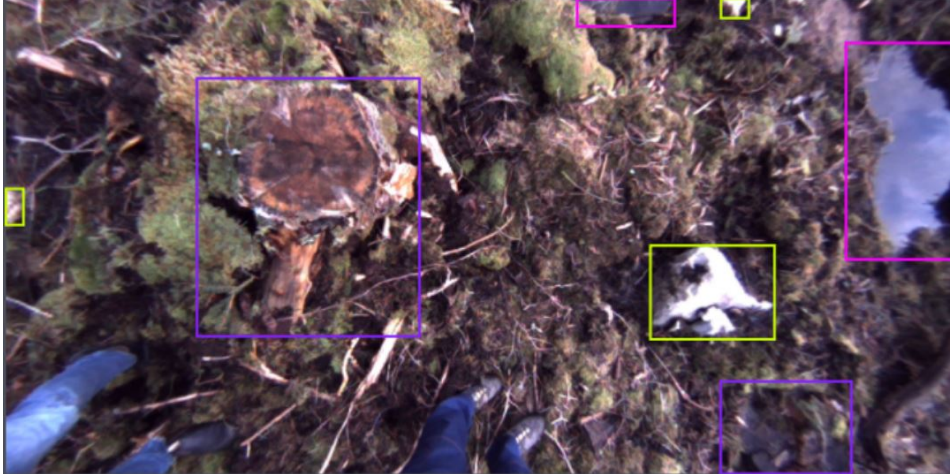
Figure 3.3: Example of an annotated image: Purple bounding boxes mark out stumps, pink bounding boxes mark out water, and yellow bounding boxes mark out stones.
