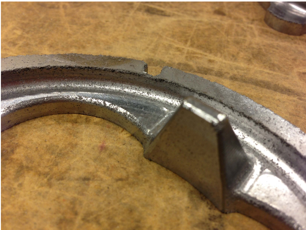
Figure 4.6: Chapped edges on one of the final stator parts
