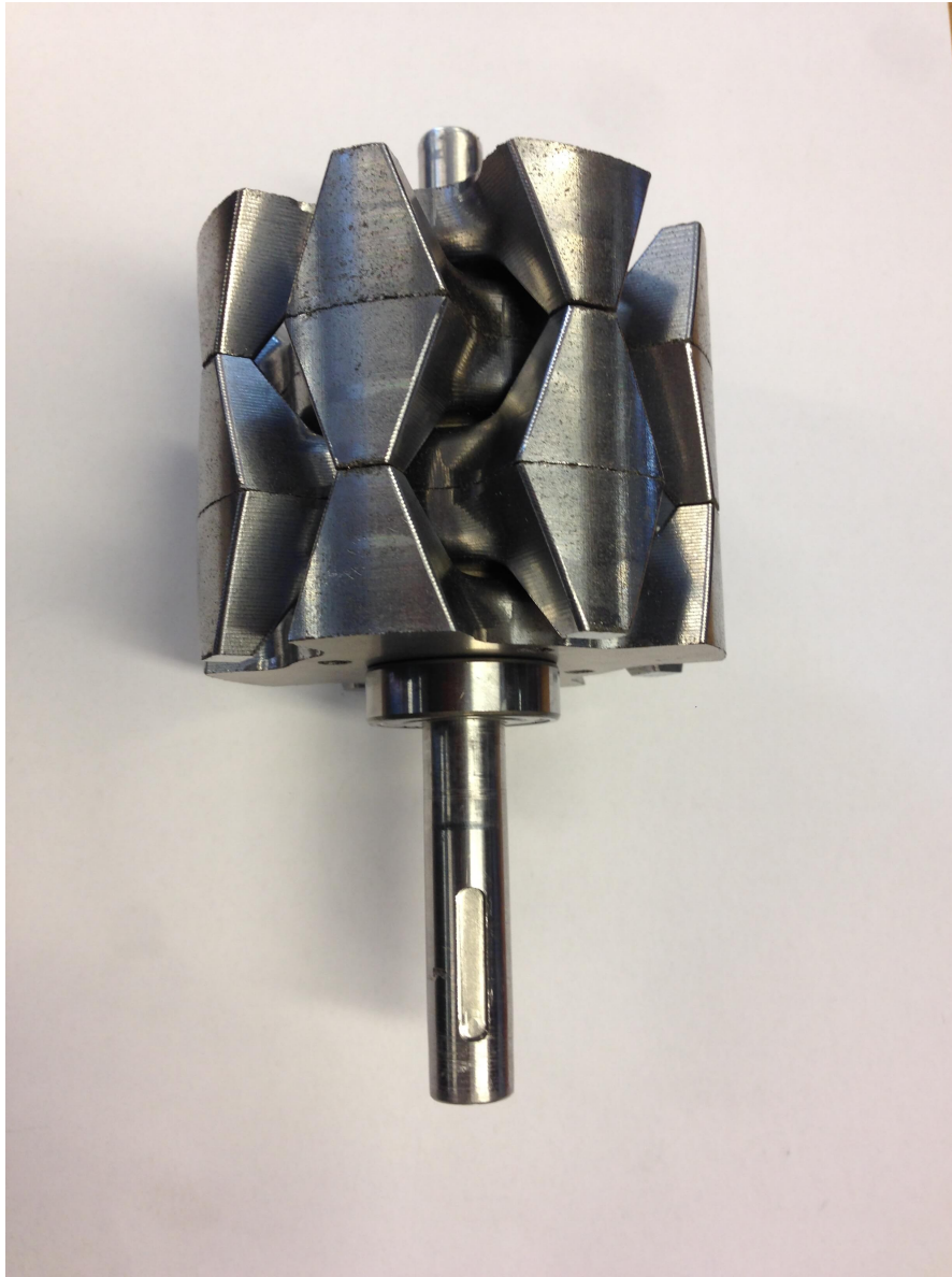
Figure 4.4: Final mounted rotor with axle and bearings
