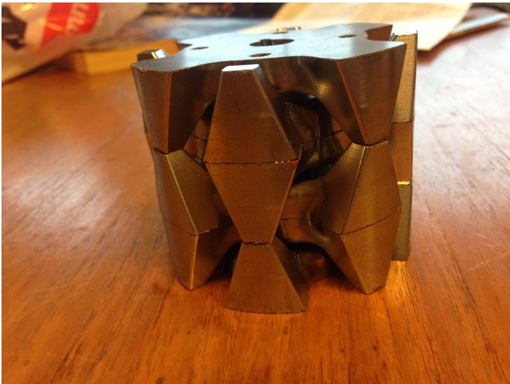
Figure 4.3: Chapped edges on final rotor parts
