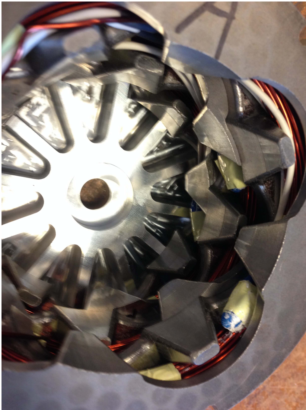
Figure 4.10: Inside of the wound stator, where the thermal switches can be seen as white/blue component taped to the winding
