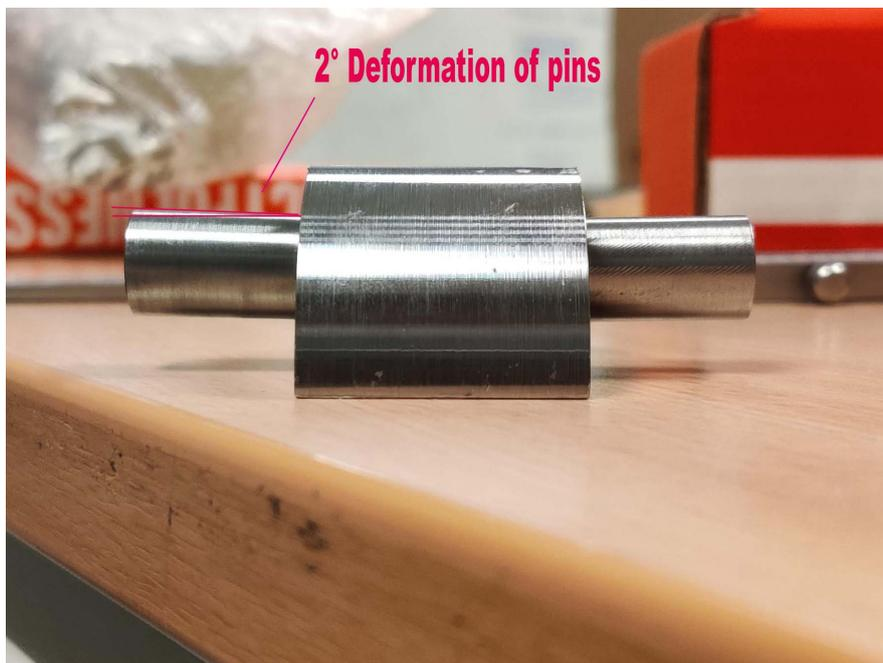
**Figure 3.25:** Picture showing the angular deformation of the pins in the split hoop fixture.
