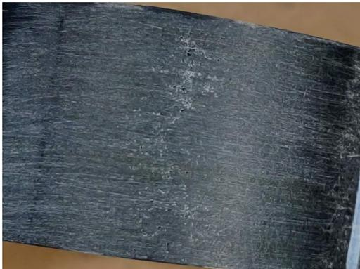
(a) Picture showing pinholes which occurred in some specimen
