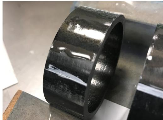
(b) Picture of Surface prepared with cured AE10 glue.
