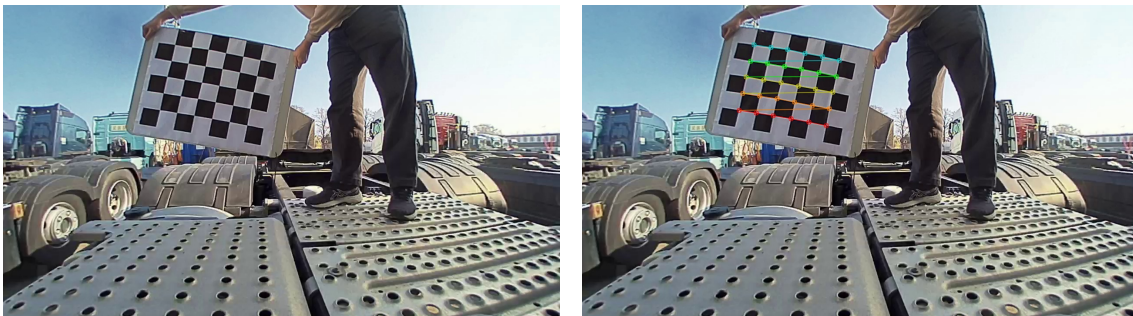
Figure 3.7: Checkerboard image before and after corner detection.
