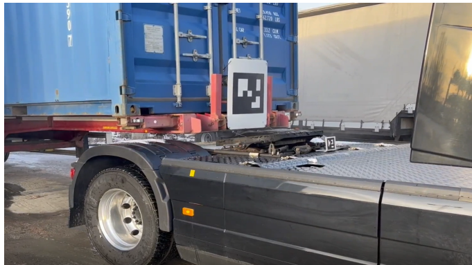
Figure 1.3: ArUco markers placed at fixed positions on the trailer and the fifth wheel.
