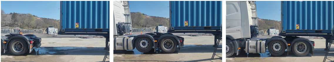
Figure 1.2: The reversing sequence for the truck and trailer coupling.
