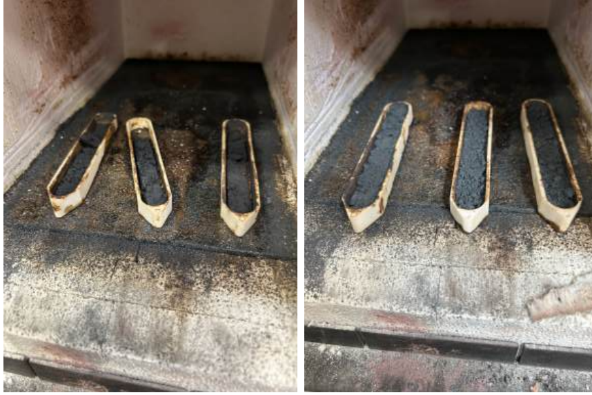
Figure A.2: 40g samples of \text{La}_{0.5}\text{Mg}_{0.5}\text{MnO}_3 and \text{Ca}_{0.56}\text{Mg}_{0.063}\text{Y}_{0.38}\text{MnO}_3 after calcination at 1300 °C, Left: \text{La}_{0.5}\text{Mg}_{0.5}\text{MnO}_3 , Right: \text{Ca}_{0.56}\text{Mg}_{0.063}\text{Y}_{0.38}\text{MnO}_3 .
