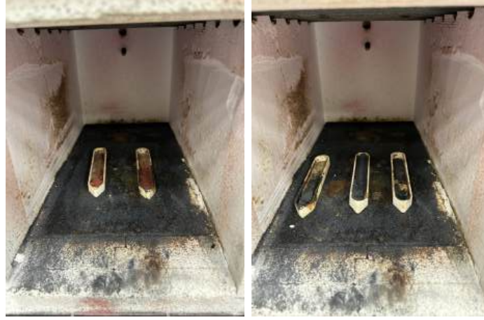
Figure 3.2: 5g samples of \text{Ca}_{0.5}\text{La}_{0.5}\text{FeO}_{3-\delta} , \text{La}_{0.5}\text{Mg}_{0.5}\text{MnO}_{3-\delta} , \text{Ca}_{0.56}\text{Y}_{0.44}\text{MnO}_{3-\delta} and \text{Ca}_{0.56}\text{Mg}_{0.063}\text{Y}_{0.38}\text{MnO}_{3-\delta} before calcination. From left to right: \text{Ca}_{0.5}\text{La}_{0.5}\text{FeO}_{3-\delta} , \text{Ca}_{0.5}\text{La}_{0.5}\text{FeO}_{3-\delta} , \text{La}_{0.5}\text{Mg}_{0.5}\text{MnO}_{3-\delta} , \text{Ca}_{0.56}\text{Y}_{0.44}\text{MnO}_{3-\delta} , \text{Ca}_{0.56}\text{Mg}_{0.063}\text{Y}_{0.38}\text{MnO}_{3-\delta} .
