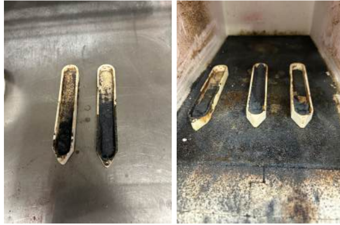
Figure 4.1: 5g samples of \text{Ca}_{0.5}\text{La}_{0.5}\text{FeO}_{3-\delta} , \text{La}_{0.5}\text{Mg}_{0.5}\text{MnO}_{3-\delta} , \text{Ca}_{0.56}\text{Y}_{0.44}\text{MnO}_{3-\delta} and \text{Ca}_{0.56}\text{Mg}_{0.063}\text{Y}_{0.38}\text{MnO}_{3-\delta} after calcination. From left to right: \text{Ca}_{0.5}\text{La}_{0.5}\text{FeO}_{3-\delta} , \text{Ca}_{0.5}\text{La}_{0.5}\text{FeO}_{3-\delta} , \text{La}_{0.5}\text{Mg}_{0.5}\text{MnO}_{3-\delta} , \text{Ca}_{0.56}\text{Y}_{0.44}\text{MnO}_{3-\delta} , \text{Ca}_{0.56}\text{Mg}_{0.063}\text{Y}_{0.38}\text{MnO}_{3-\delta} .
