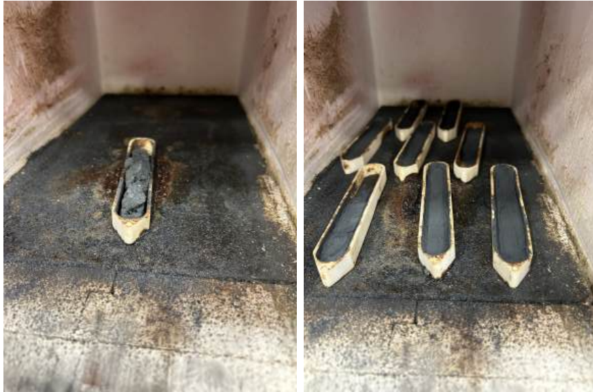
Figure A.1: 30-40 g samples of \text{Ca}_{0.5}\text{La}_{0.5}\text{FeO}_3 , \text{La}_{0.5}\text{Mg}_{0.5}\text{MnO}_3 , \text{Ca}_{0.56}\text{Y}_{0.44}\text{MnO}_3 and \text{Ca}_{0.56}\text{Mg}_{0.063}\text{Y}_{0.38}\text{MnO}_3 after calcination at 1250 °C. Left: \text{Ca}_{0.5}\text{La}_{0.5}\text{FeO}_3 . Right: from back to front \text{La}_{0.5}\text{Mg}_{0.5}\text{MnO}_3 , \text{Ca}_{0.56}\text{Y}_{0.44}\text{MnO}_3 , \text{Ca}_{0.56}\text{Mg}_{0.063}\text{Y}_{0.38}\text{MnO}_3 .
