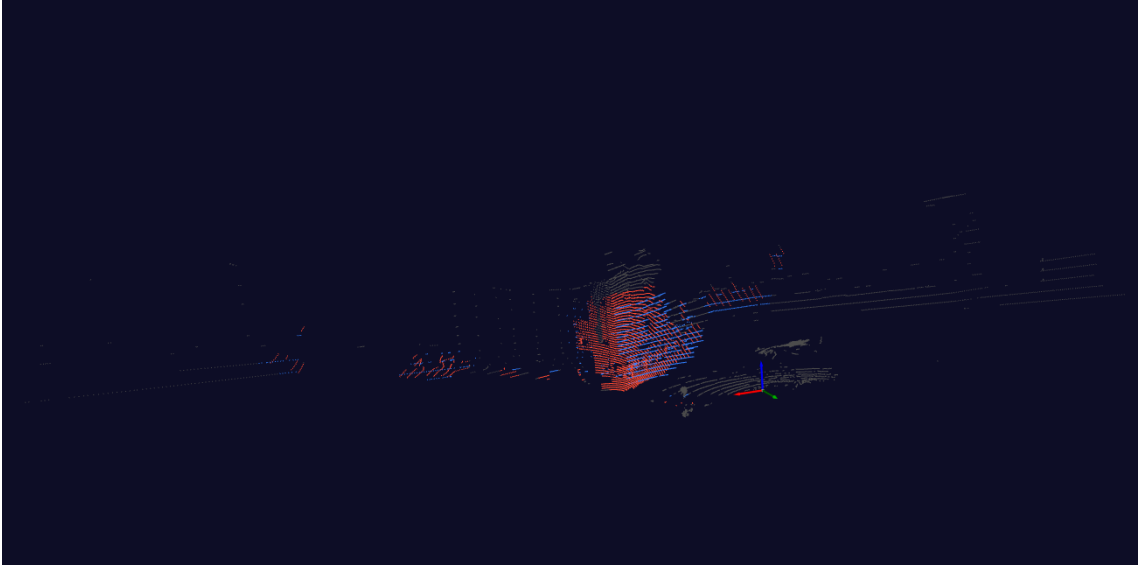
Figure 4.24: Overlap detection result. Red: Airy points in the overlap region. Blue: Helios points in the overlap region. Gray: discarded non-overlapping points. The overlap radius threshold was 1.2 m.
