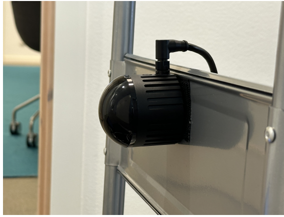
Figure 3.12: Close-up of the LiDAR sensor mounted on the cart for Step 2. The dome faces the front of the cart and the cable points upward, giving an expected yaw offset of 0^\circ \pm 3^\circ .
