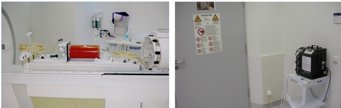
Figure 3.18: The complete setup for measurement with body coil MR scanner. Phantom setup with MR scanner on the left and the water pump and temperature regulator on the right.
